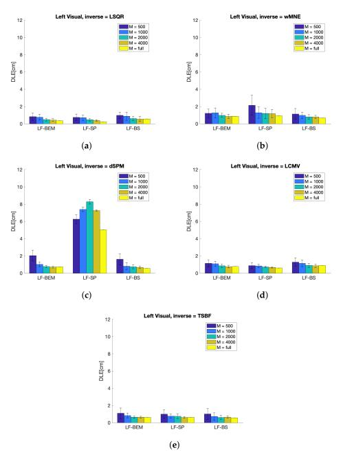
**Figure 4.** Left Visual evoked field: Mean DLE [cm] and standard deviation obtained averaging over N = 10 runs using LSQR (a), wMNE (b), dSPM (c), LCMV (d), and TSBF (e) at 90 ms for LF-BEM, LF-SP, and LF-BS.
