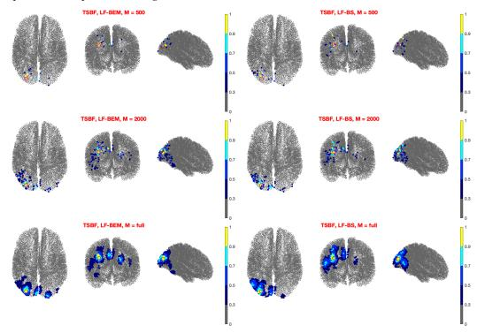
**Figure 15.** Right Visual evoked field: The intensity of the estimated sources, averaged over N = 10 runs, at 90 ms obtained using TSBF with M = 500 random points (first row), M = 2000 (second row) and the full source space (third row) for LF-BEM (left column) and LF-BS (right column). The red circle represents the dipole fitted using MNE.
