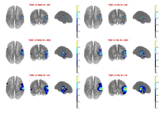
**Figure 10.** Left Auditory evoked field: The intensity of the estimated sources, averaged over N = 10 runs, at 90 ms obtained using TSBF with M = 500 random points (first row), M = 2000 (second row) and the full source space (third row) for LF-BEM (left column) and LF-BS (right column). The red circle represents the dipole fitted using MNE.
