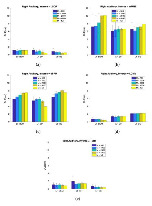
**Figure 3.** Right Auditory evoked field: Mean DLE [cm] and standard deviation obtained averaging over N = 10 runs using LSQR (**a**), wMNE (**b**), dSPM (**c**), LCMV (**d**), and TSBF (**e**) at 90 ms for LF-BEM, LF-SP, and LF-BS.
