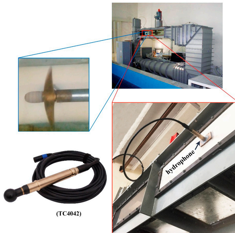
Figure 10. Arrangement of TC4042 hydrophone on cavitation tunnel.
