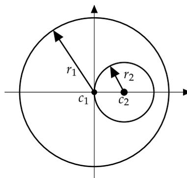
**Figure 4.** Domain on which an exact solution is computed. The outer boundary is the unit circle. The inner boundary is the circle of center  $c_2 = 0.4$  and of radius  $r_2 = 0.4$ . The Dirichlet boundary conditions used are such that the value is  $c_1 = 0$  on the inner boundary and  $r_1 = 1$  on the outer boundary.
