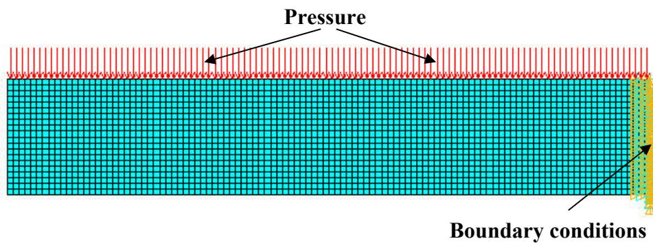
Figure 3 Finite element model of the composite beam
