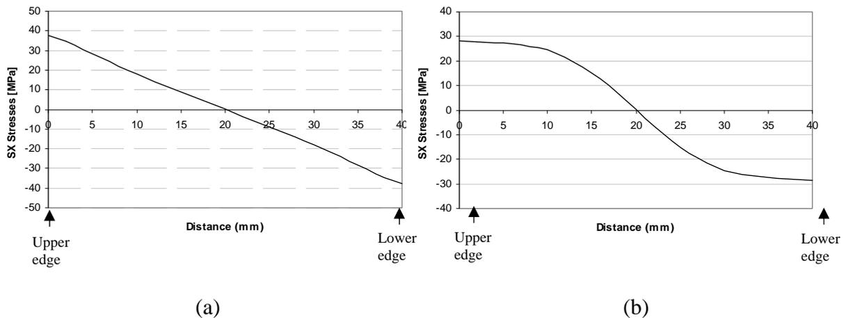
**Figure 4** The distribution of the  $\sigma_x$  stress component in the elastic (a) and elastic-plastic (b) solutions along the section of the beam at 200 mm for  $0^\circ$  orientation
