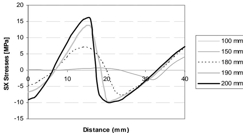
**Figure 7** Residual stress component ( $\sigma_x$ ) of the composite beam with  $[15]_2$  orientation
