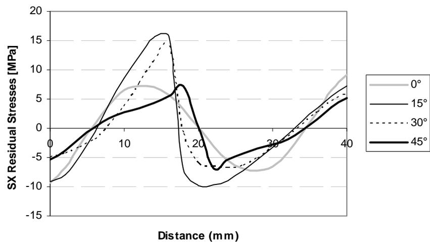
**Figure 15** Residual stress component ( $\sigma_x$ ) of the composite beam for 200 mm
