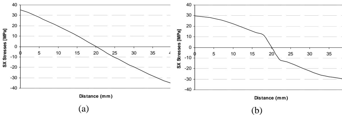
**Figure 9** The distribution of the  $\sigma_x$  stress component in the elastic (a) and elastic-plastic (b) solutions along the section of the beam at 200 mm for  $45^\circ$  orientation
