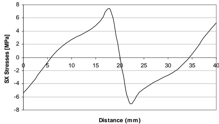
**Figure 10** Residual stress component ( $\sigma_x$ ) of the composite beam with  $[45]_2$  orientation for 200 mm
