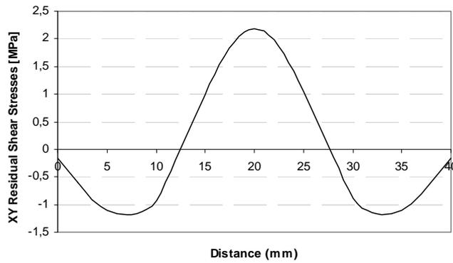
**Figure 12** Residual stress component ( $\tau_{xy}$ ) of the composite beam with  $[0]_2$  orientation for 200 mm
