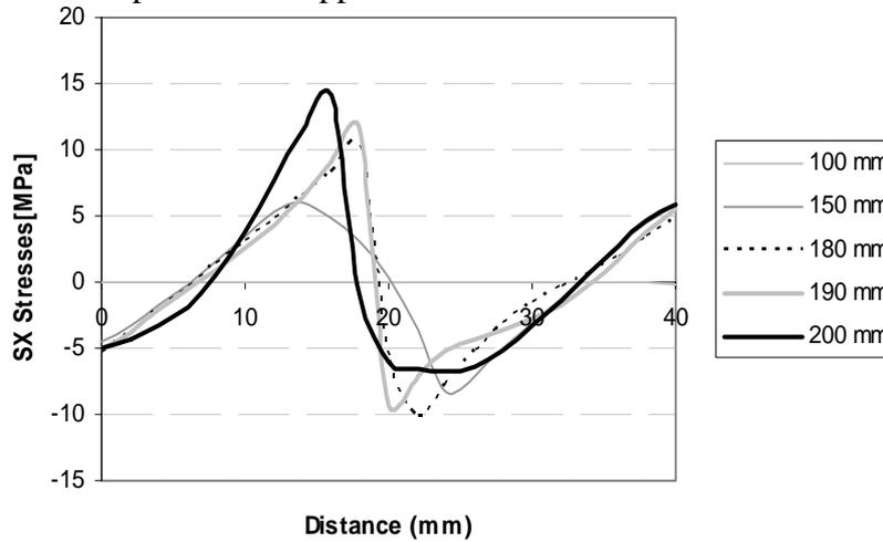
**Figure 8** Residual stress component ( $\sigma_x$ ) of the composite beam with  $[30]_2$  orientation
