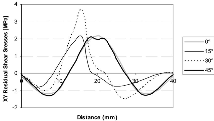
**Figure 14** Residual stress component ( $\tau_{xy}$ ) of the composite beam for 200 mm
