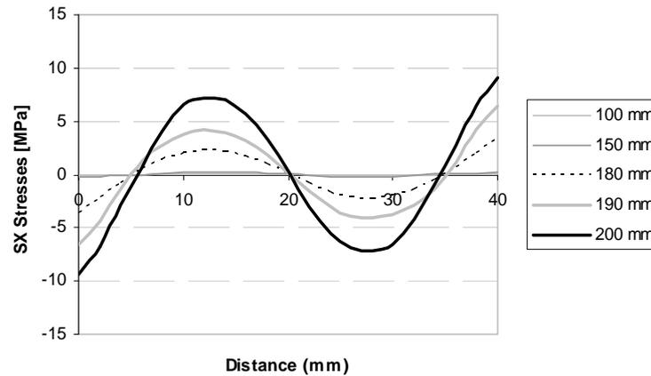
**Figure 6** Residual stress component ( $\sigma_x$ ) of the composite beam with  $[0]_2$  orientation
