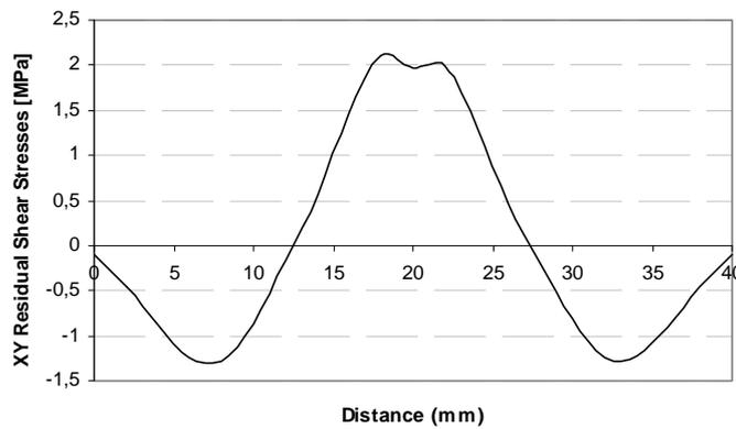
**Figure 13** Residual stress component ( $\tau_{xy}$ ) of the composite beam with  $[45]_2$  orientation for 200 mm
