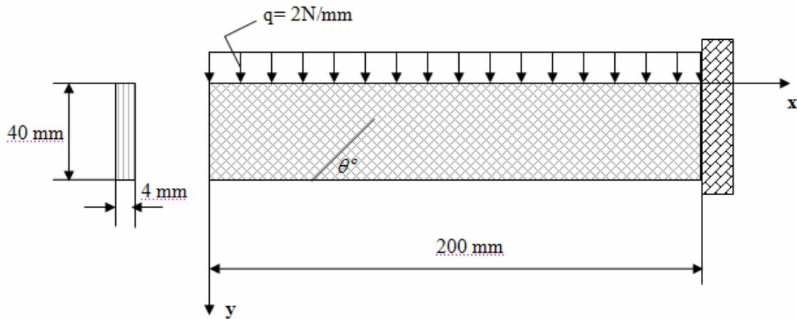
**Figure 1** Schematic view of the cantilever composite beam under uniform loading of 2 N/mm
