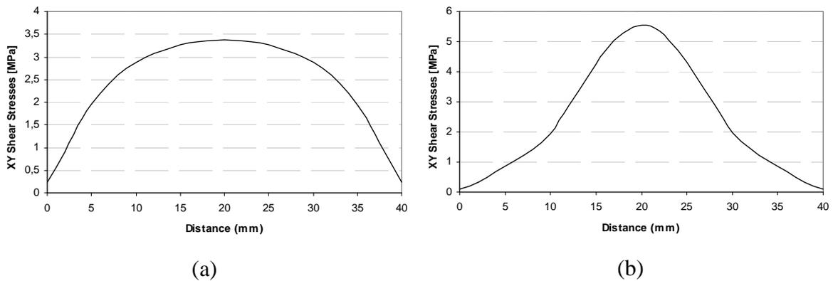
**Figure 11** The distribution of  $\tau_{xy}$  along the section of the beam oriented  $0^\circ$  at the fixed end, for the elastic (a) and plastic (b) solutions
