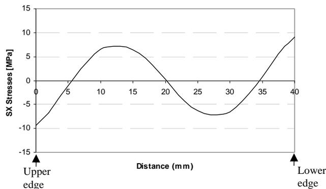
**Figure 5** Residual stress component ( $\sigma_x$ ) of the composite beam with  $[0]_2$  orientation for 200 mm
