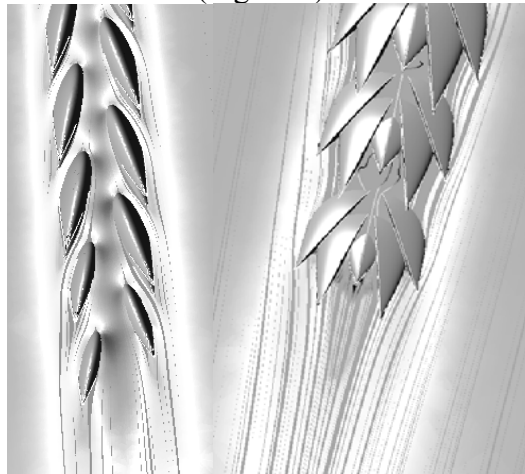
Figure 3. Streamlines and eddies for bread wheat spike
