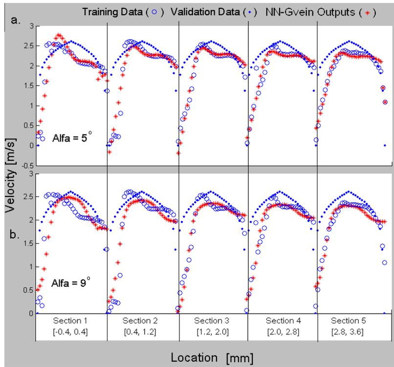
Figure 7. Velocity profiles in the AV graft-to-vein connection for  $\alpha = 5^\circ$  and  $\alpha = 9^\circ$
