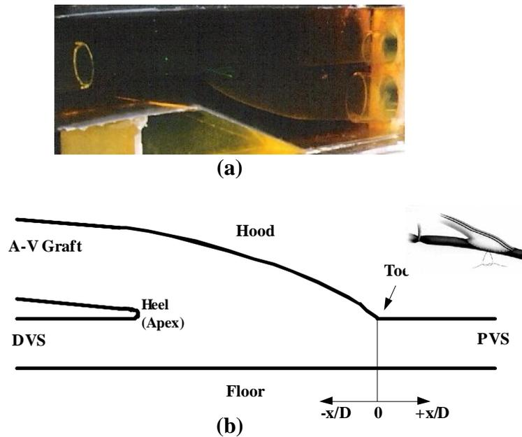
**Figure 1.** (a) 3D view, (b) bifurcation plane geometry and nomenclature of the AV graft to vein connection model
