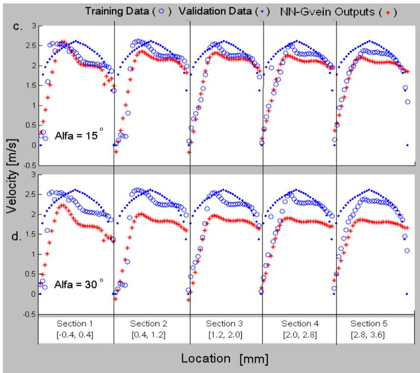
Figure 8. Velocity profiles in the AV graft-to-vein connection for  $\alpha = 15^\circ$  and  $\alpha = 30^\circ$
