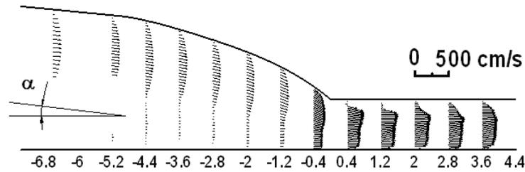
**Figure 4.** Velocity profiles of blood stream flow in graft-to-vein connection
