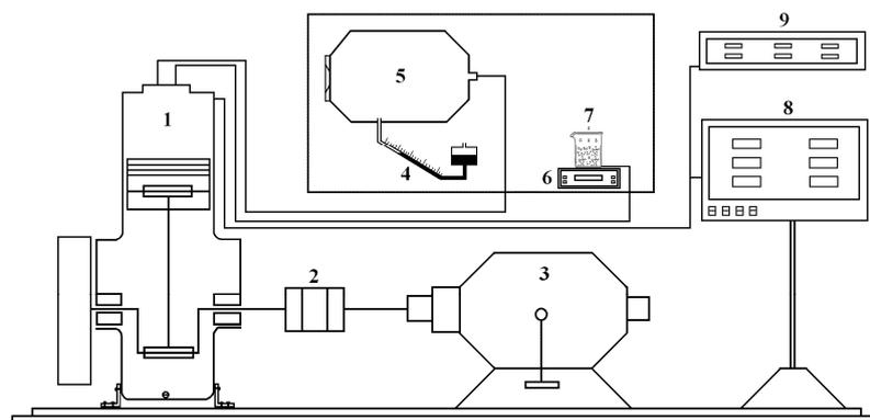
Fig. 2. Schematic view of the engine test bed (1- Engine, 2- Clutch, 3- Dynamometer, 4- Manometer, 5- Air tank, 6- Digital scale, 7- Fuel tank, 8- Exhaust gas analyzer, 9- Smoke meter).
