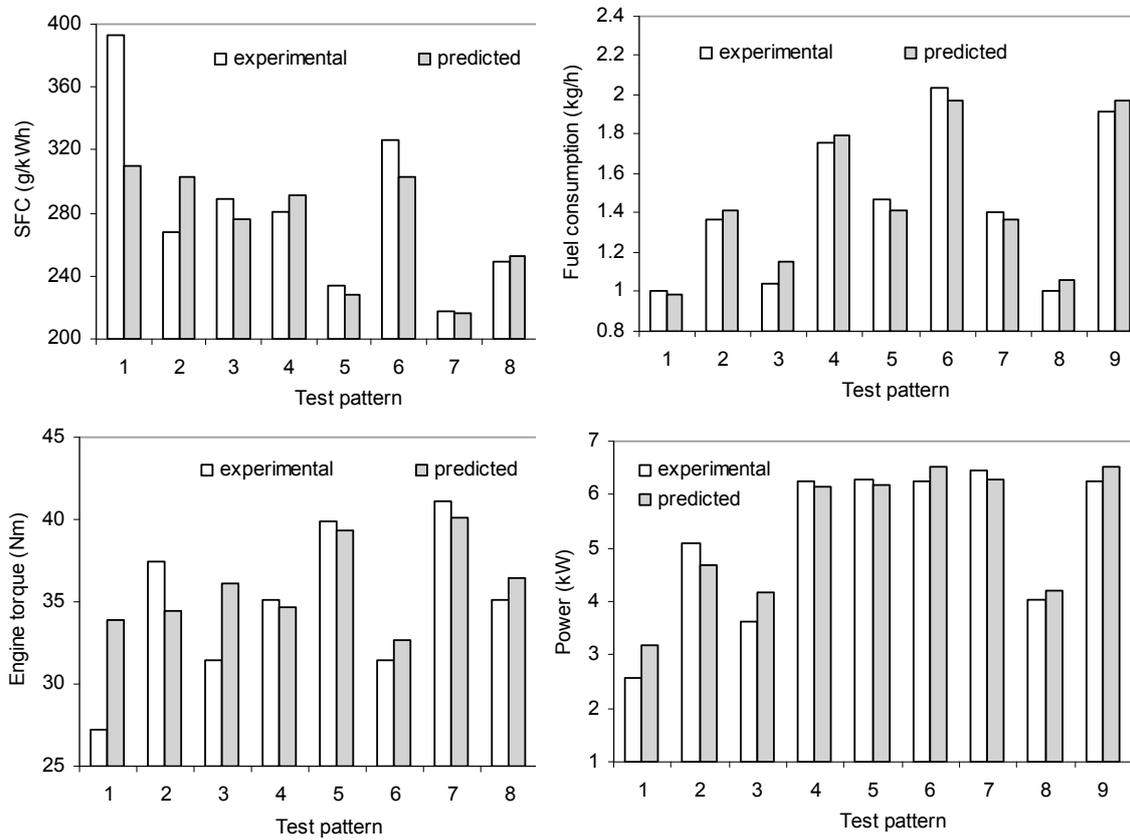
Fig. 4. Experimental and ANN predicted results of engine performance.
