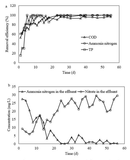
**Figure 2.** Pollutant concentration variation and removal efficiency. (**a**) the pollutant removal efficiency; (**b**) concentration variation of ammonia and nitrate in the effluent.
