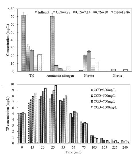
Figure 3. Effects of different organic loadings on COD removal, ammonia nitrogen removal, total nitrogen removal and phosphorus removal (the OLR unit is kg  $COD/m^3 \cdot d$ ). (a) pollutant removal efficiency; (b) pollutant concentration in the effluent; (c) TP concentration variation in the effluent with the variation of influent COD.
