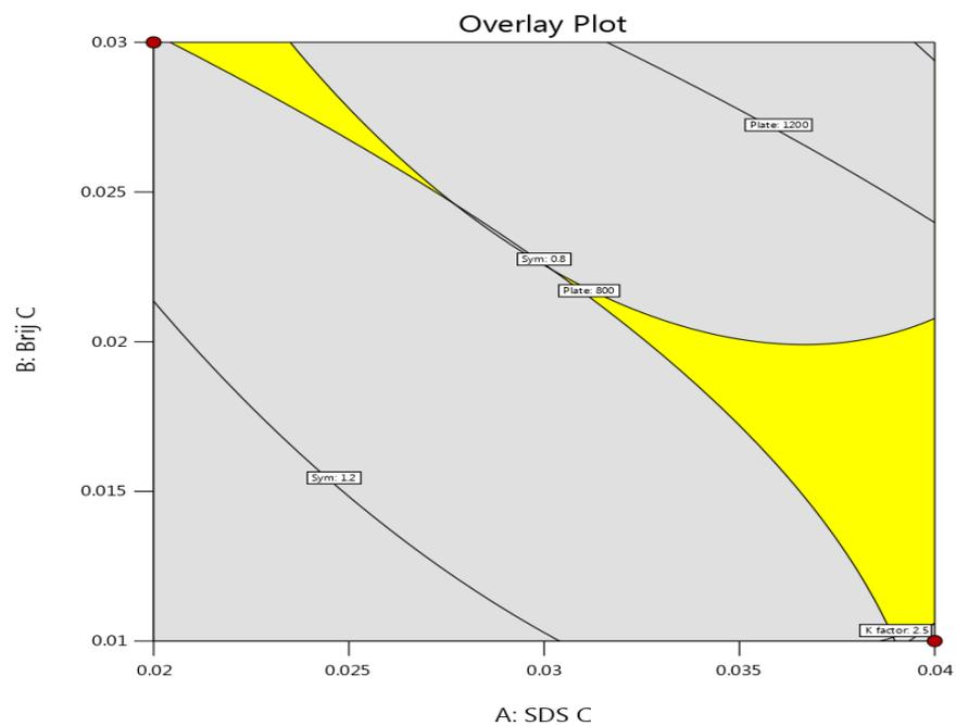
Figure 4. Overlay plot displaying the preferred responses within the appropriate parameters (sweet spot).
