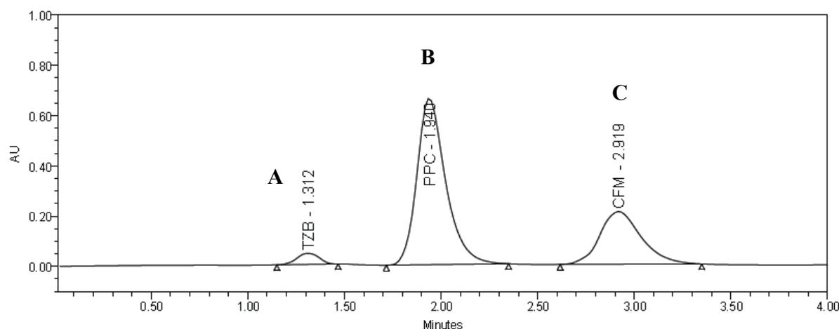
**Figure 5.** Chromatogram showing separation of (A) TZB, (B) PPC and (C) CFM in a laboratory-prepared mixture under the chromatographic parameters for validation. Mobile phase: 15 mM Brij-35, 38 mM SDS, pH 3.5 at one mL per min of flow rate.
