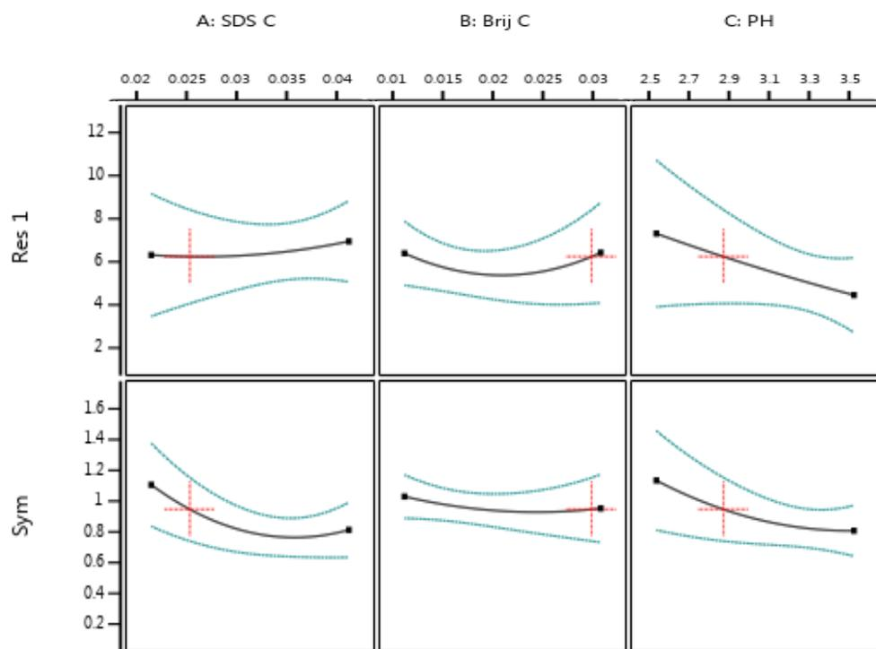
**Figure 2.** Plots of perturbation illustrating the impact of the parameters under study on resolution between the analytes and the symmetry factors of the peak (Black lines, result line; Green lines, upper and lower confidence intervals).
