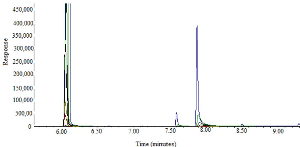
**Figure 6.** Overlaid GC-MS spectra of standard FCO and TOH at different concentrations.
