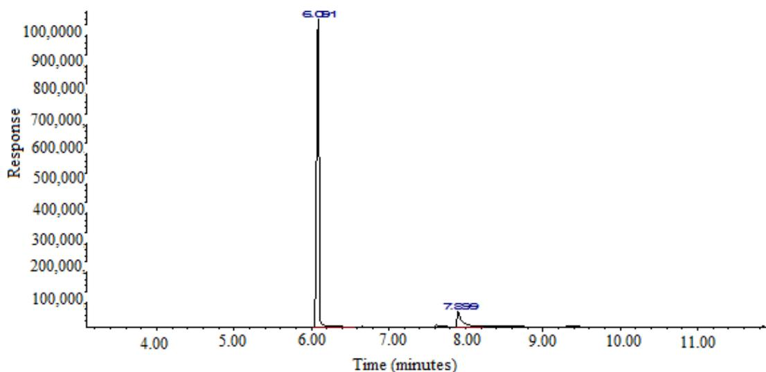
**Figure 5.** Gas chromatography–mass spectrometry (GC-MS) peaks of standard FCO (*R*<sub>t</sub> = 6.091 min) and TOH (*R*<sub>t</sub> = 7.889 min).
