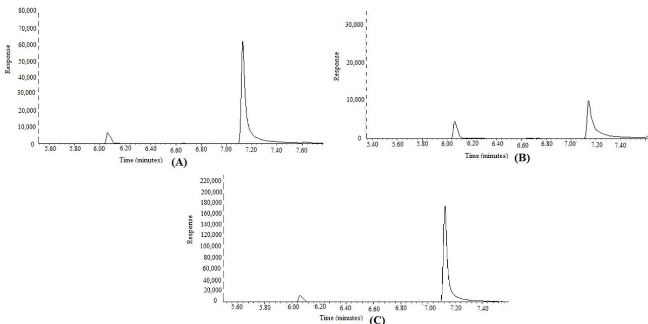
**Figure 7.** Representative GC-MS peaks of FCO and TOH in methanolic extracts of *F. vulgare* obtained from (A) IND, (B) PAK, and (C) SA.
