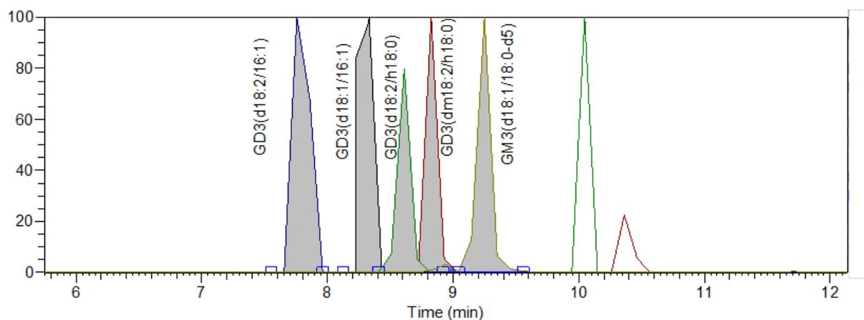
**Figure 5.** LC-MS/MS chromatogram for disialoganglioside GD3 species containing three different sphingoid bases (d18:1, d18:2, dm18:2) and both hydroxylated and non-hydroxylated fatty acids. GM3 internal standard is included as elution time reference. Comparison of retention times is not straightforward due to the different fatty acids attached, but GD3 species elute as a group before the GM3 internal standard.
