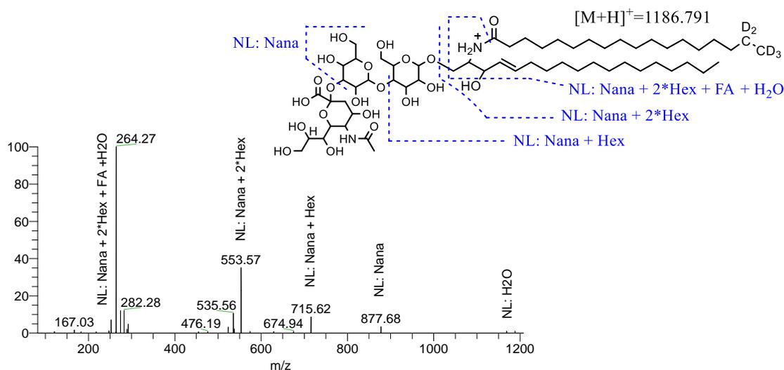
**Figure 2.** Structure and fragmentation of the deuterated GM3(d18:1/18:0-d5) standard. Schematic representation of the molecular structure and cleavage sites. Annotation is based on the corresponding neutral losses (NL) of different parts of the structure generating fragment ions.
