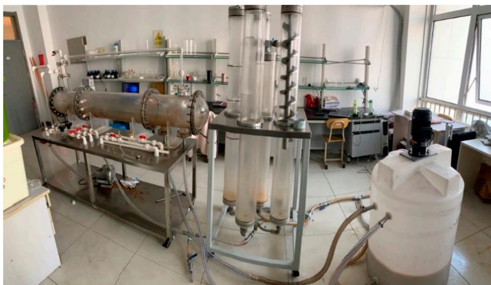
**Figure 1.** Proposed multistage multiphase oil–water separation system.
