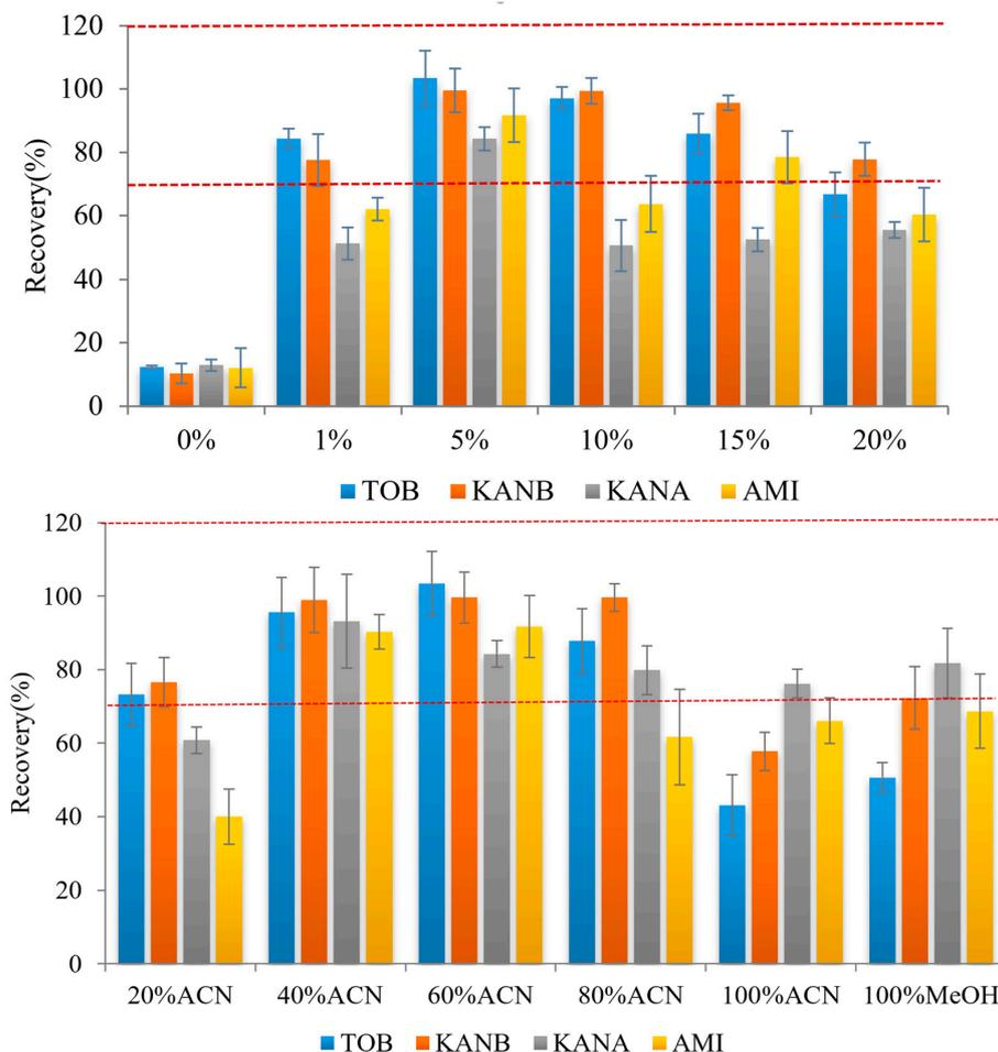
**Figure 4.** Effect on analyte recoveries of formic acid (top) and ACN content (bottom) in the elution mixture ( $n = 3$ ) (Red dash lines represents the recoveries form 70% to 120%).
