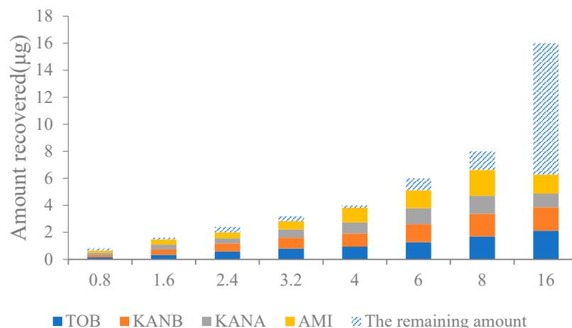
**Figure 5.** Effect on analyte recoveries of the capacity of AAC column.
