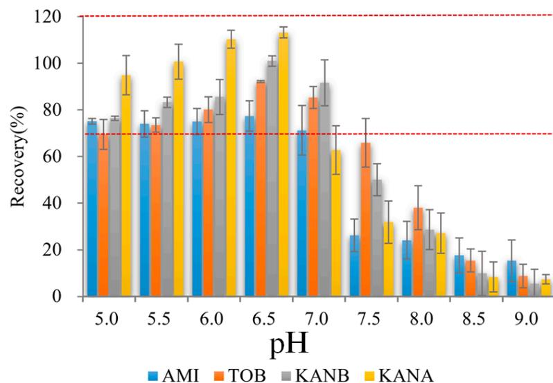
**Figure 3.** Effect on analytes recoveries of binding buffer pH ( $n = 3$ ) (Red dash lines represents the recoveries form 70% to 120%).
