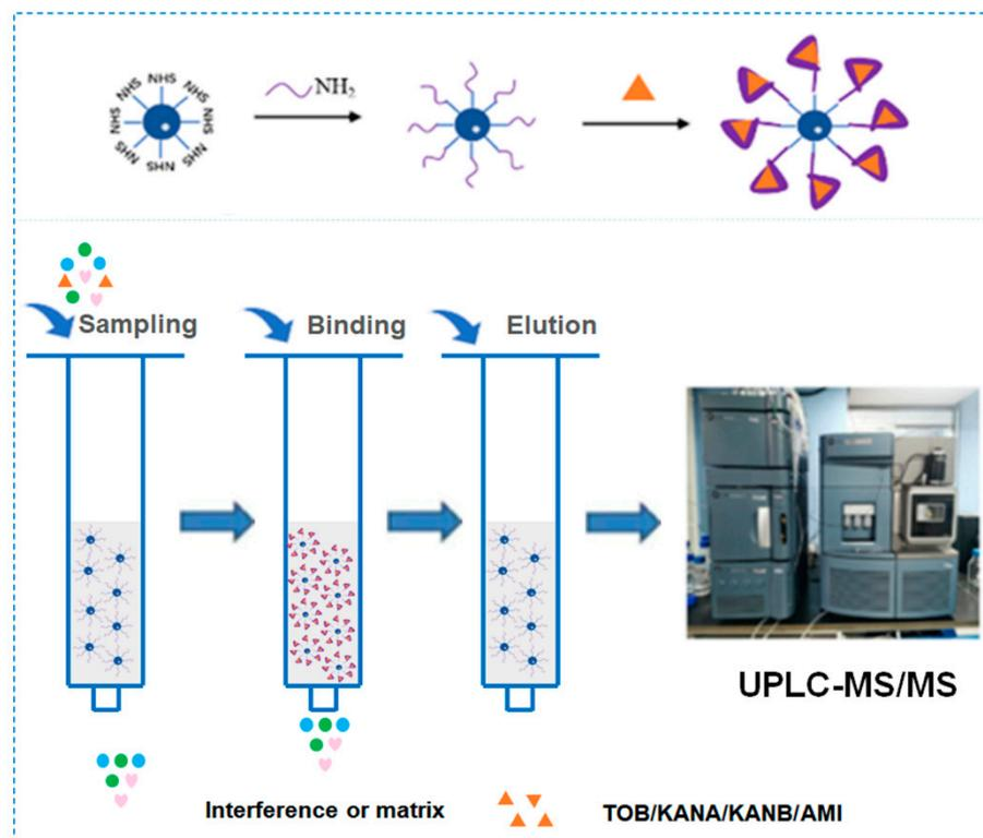
**Figure 1.** Schematic diagram of aptamer and agarose coupling and AAC working principle.
