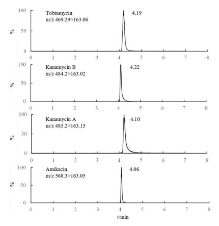
**Figure 2.** MRM chromatograms of 4 Ags (1  $\mu$ g/mL).
