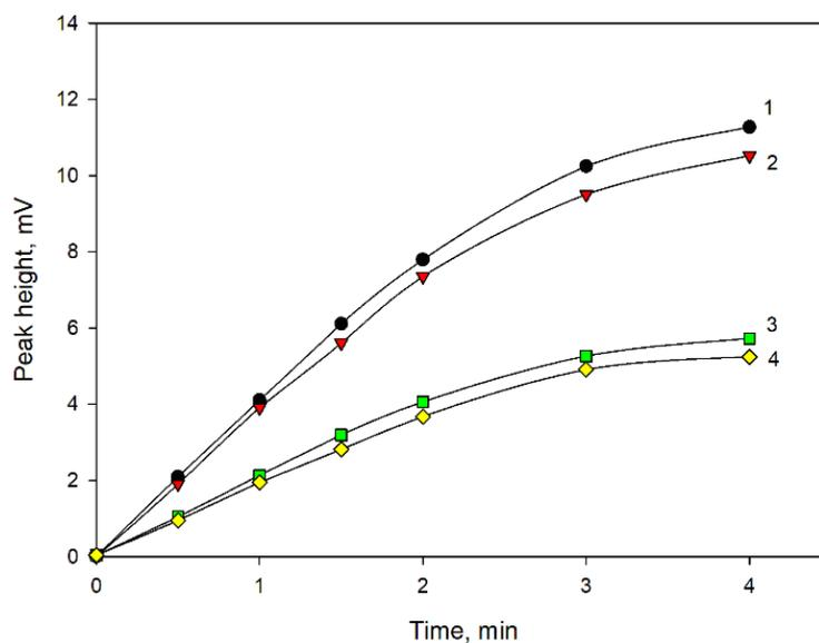
**Figure 2.** Dependencies of peak heights of toluene (1, 3) and benzene (2, 4) in dynamic HSA obtained for a series of model solutions at flow rates of 15 mL/min (3, 4) and 30 mL/min (1, 2).
