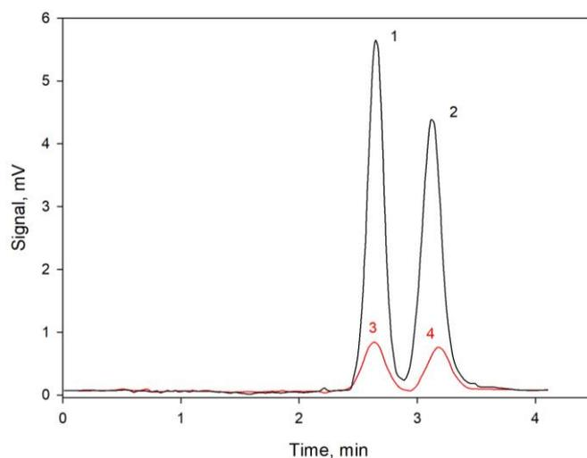
**Figure 4.** GC determination of benzene (1, 3) and toluene (2, 4) in a model solution (5 mg/L) with preconcentration by a selective adsorption of the gas-extractant (1, 2) and without it (3, 4). CO<sub>2</sub> flow rate—30 mL/min, time—2 min. Separation column—Chromaton N-AW (60–80 mesh) coated with 5% OV-17.
