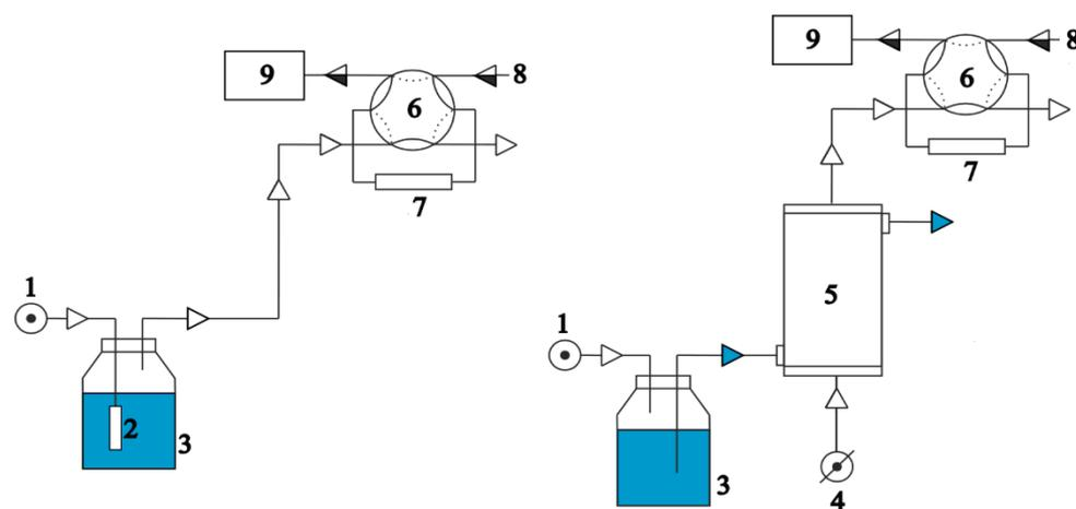
**Figure 1.** Schematic diagrams of the experimental setup used for dynamic HSA (left) and for continuous chromatomembrane HSA (right) with absorption of the gas extractant in both cases. 1: carrier gas flow regulator; 2: gas sparger; 3: sample vessel with an aqueous solution of VOCs; 4: gas-extractant flow regulator; 5: chromatomembrane cell; 6: switching valve; 7: CO<sub>2</sub> absorbing cartridge; 8: inlet for the carrier gas; 9: gas chromatograph.
