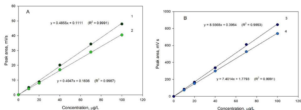
**Figure 6.** Peak area of dependencies on preconcentrations of aliphatic (A) and aromatic (B) hydrocarbons found by using dynamic gas extraction combined with capillary GC. 1—benzene, 2—toluene, 3—n-hexane, and 4—n-heptane.
