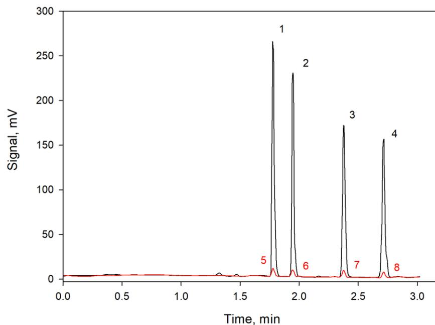
**Figure 5.** Gas chromatograms obtained with capillary GC column used for the determination of n-hexane (1, 5), benzene (2, 6), n-heptane (3, 7) and toluene (4, 8) in a model solution after preconcentration via selective adsorption of the gas-extractant (1, 2, 3, 4) and without it (5, 6, 7, 8). Concentrations of n-hexane and n-heptane—0.2 mg/L; benzene and toluene—5 mg/L. CO<sub>2</sub> flow rate—30 mL/min, time—2 min. Fused silica column with dimethylpolysiloxane coating.
