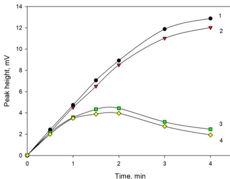
**Figure 3.** Dependencies of peak heights of n-heptane (2, 4) and n-hexane (1, 3) on the passing time of the gas-extractant (30 mL/min) through aqueous solution in the case of chromatomembrane (1, 2) and dynamic HSA (3, 4).
