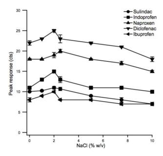
**Figure S2.** Effect of addition of salt on peak responses using mixed matrix membrane tip microextraction. Extraction parameters: sample pH 3.5; sample volume, 10 mL; desorption solvent volume, 40  $\mu$ L; analyte concentration, 100 ng L<sup>-1</sup> of spiked solution. (Error bars represent standard deviations of results, *n* = 3).
