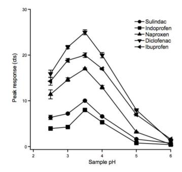
**Figure S1.** Effect of sample pH on peak responses using mixed matrix membrane tip microextraction. Extraction parameters: addition of salt, 2% (w/v); sample volume, 10 mL; desorption solvent volume, 40  $\mu$ L; analyte concentration, 100 ng L<sup>-1</sup> of spiked solution. (Error bars represent standard deviations of results, *n* = 3).
