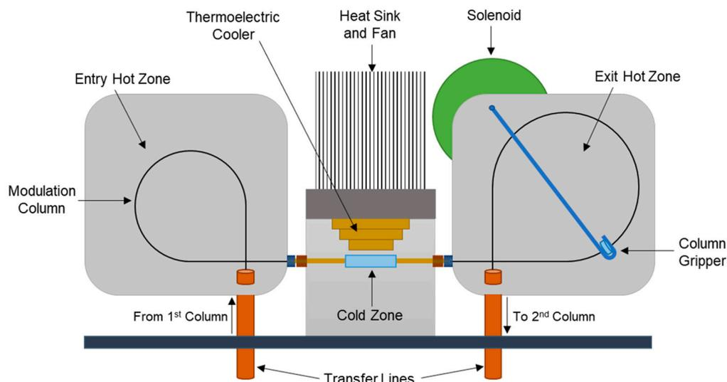
**Figure 1.** Schematic of the solid-state modulator, based on Reference [13].
