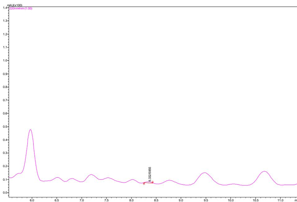
**Figure S3.** HPLC-UV chromatogram of a standard solution of oxalic acid at 20 µg/mL.
