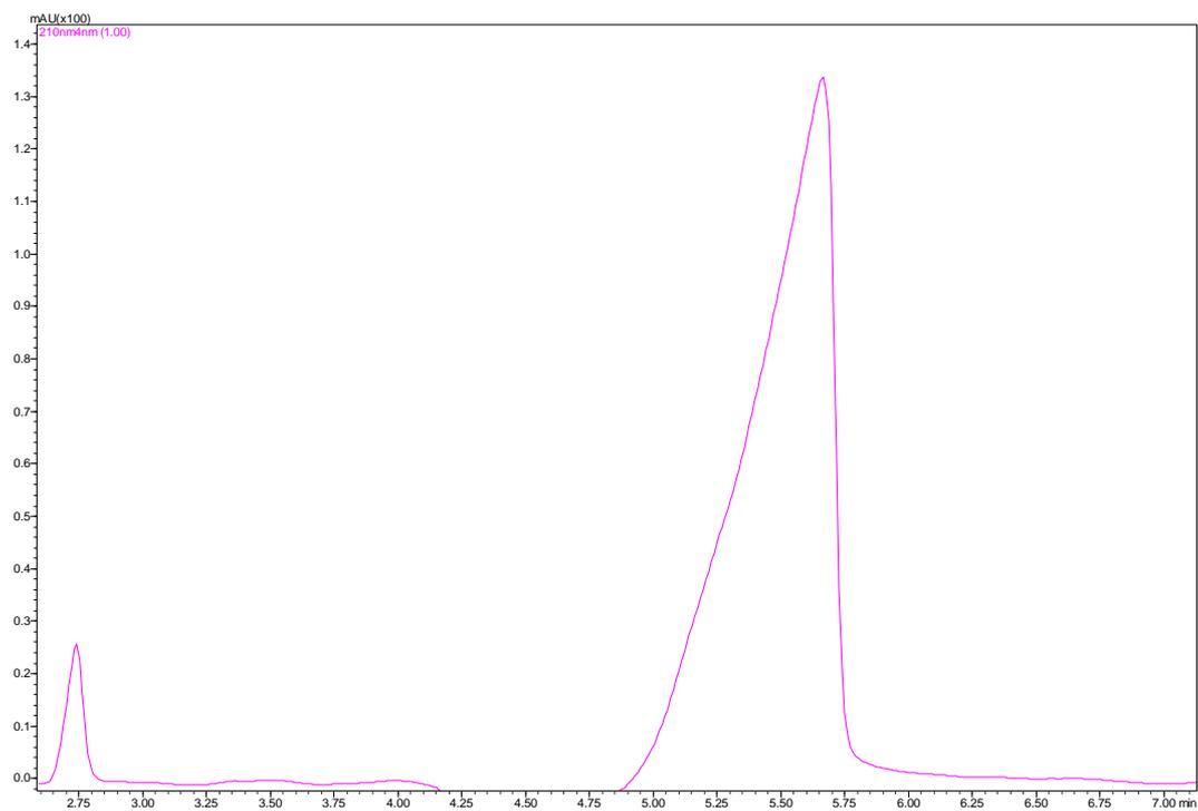
**Figure S10.** HILIC-ESI/MS SIM chromatogram of LA and OA in standards solution mix (using ammonium acetate buffer)
