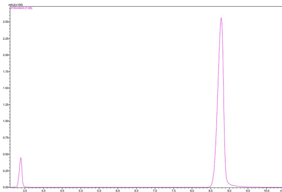
**Figure S9.** HILIC-PDA chromatogram of LA and OA in standards solution mix (using ammonium acetate buffer)
