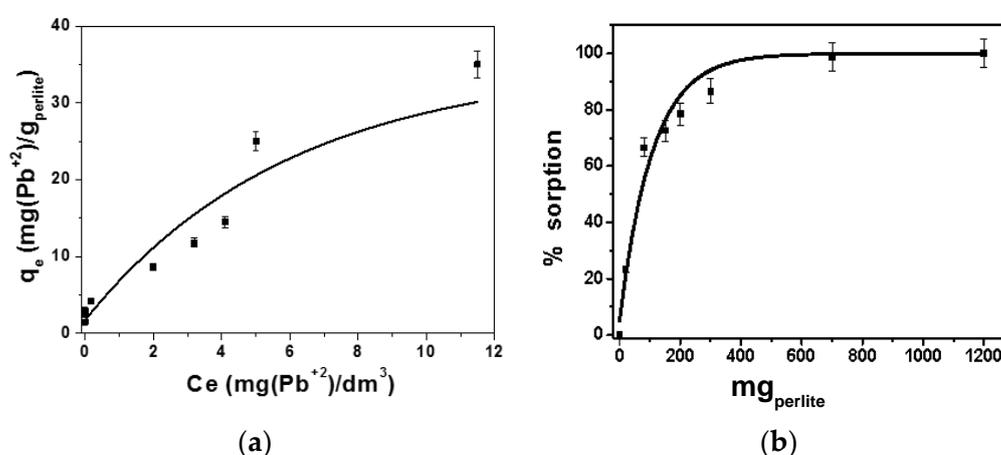
**Figure 2.** (a) Single batch test in de-mineralized water for lead ion retention on perlite (1–2 mm bead size, 80 rpm, 15 mg(Pb<sup>+2</sup>)/dm<sup>3</sup>, 298 K); (b) effect of perlite dosage on the sorption.
