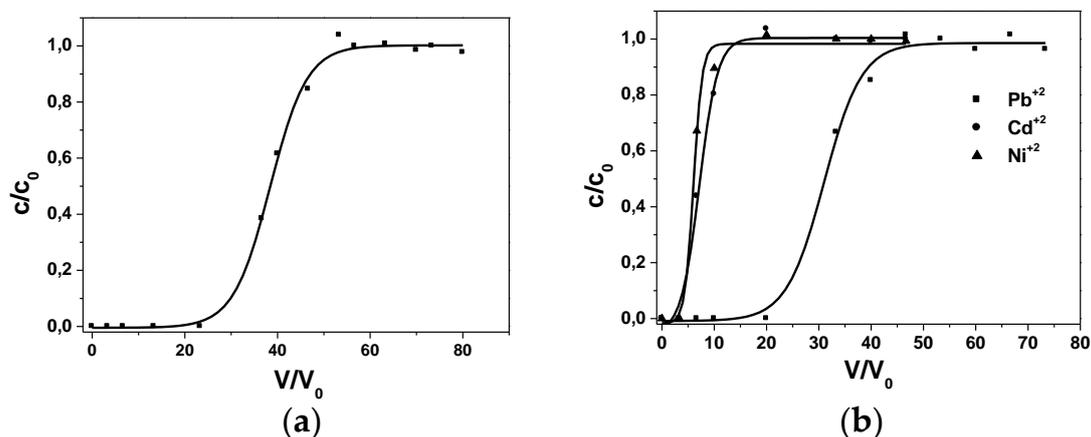
**Figure 4.** Breakthrough curves in de-mineralized water for (a) lead ions and (b) solution of lead, cadmium and nickel ions on perlite (1–2 mm particle size, 0.3 L/h, 15 mg(Me<sup>+2</sup>)/dm<sup>3</sup>, pH = 6, T = 298 K).
