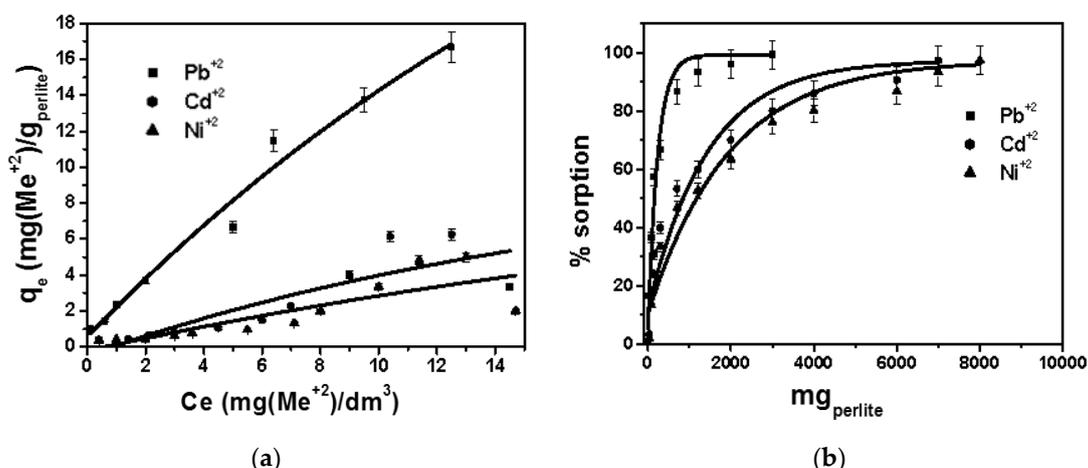
**Figure 3.** (a) Batch tests in de-mineralized water for a solution of lead, cadmium and nickel ions on perlite (1–2 mm bead size, 80 rpm, 15 mg(Me<sup>+2</sup>)/dm<sup>3</sup>, 298 K); (b) effect of perlite dosage on the sorption.
