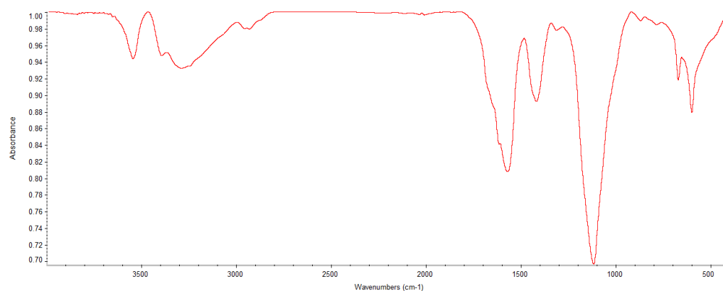
Figure 3. FTIR spectrum of polysaccharide samples from P. depressa . The abscissa and y-axis were absorbance and wavenumbers ( \text{cm}^{-1} ), respectively.
