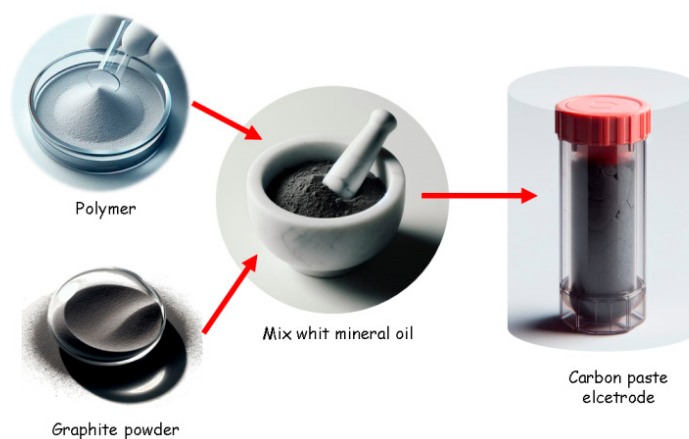
Scheme 2. Modified carbon-paste elaboration procedure.
