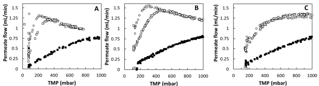
Figure 2. TMP excursion for 30 kDa and 100 kDa MWCO Hydrosart® and PES membranes. Feed flow rate of (A) 35.4 mL·min<sup>-1</sup>, (B) 59 mL·min<sup>-1</sup>, and (C) 75 mL·min<sup>-1</sup>. Empty circles represent the 100 kDa MWCO Hydrosart® membrane, full black squares represent the 30 kDa PES membrane and empty squares represent the 100 kDa PES membrane.
