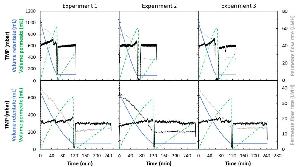
**Figure 4.** Profiles of permeate flow rate (grey dashed line), TMP (full black line), volume of retentate (blue full line), and volume of permeate (green dashed line) as a function of process time, obtained for the 100 kDa PES Sartocor<sup>®</sup> Slice 200 flat sheet cassette (upper panels) and the 100 kDa PES hollow fiber (bottom panels). Three independent experiments were performed.
