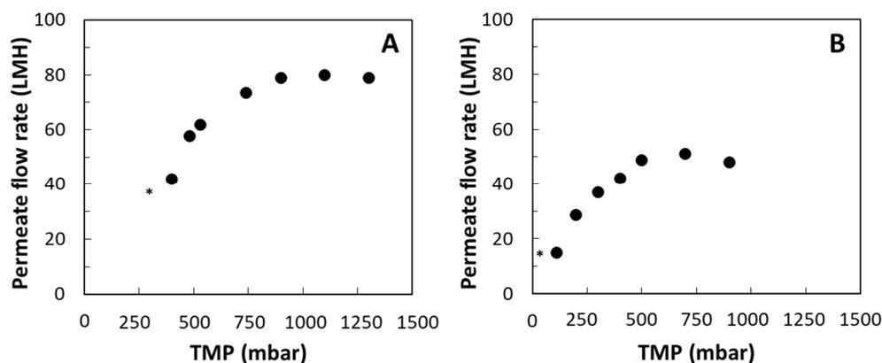
**Figure 3.** TMP excursion for 100 kDa MWCO PES Sartoco<sup>®</sup> Slice 200 flat sheet cassette vs. 100 kDa MWCO hollow fiber. (A) Feed flow rate of 260 mL/min in flat sheet cassette and (B)  $8000\text{ s}^{-1}$  shear rate (212 mL/min) in hollow fiber. \* Minimum TMP value obtained at used feed flow rate with totally opened retentate valve.
