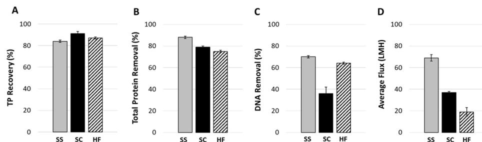
**Figure 5.** Total particle recovery (A), total protein removal (B), DNA removal (C), and average flux (D) for the 100 kDa PES Sartocor<sup>®</sup> Slice 200 flat sheet cassette vs. the 100 kDa PES hollow fiber. Full grey bars represent Ambr<sup>®</sup> CF 10 cm<sup>2</sup> (SS), full black bars represent Sartocor<sup>®</sup> Slice 200 180 cm<sup>2</sup> (SC), and dashed bars represent the hollow fiber device (HF).
