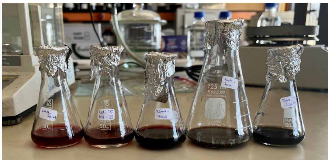
Figure S3. Color development of different molar ratios: from left to right: 5-CQA:TRP 1mM-5mM, 1mM-3,5mM, 3,5mM-7mM, 7mM-7mM and 7mM-3,5mM
