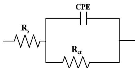
**Figure 4.** The suitable equivalent circuit used to fit EIS data.
