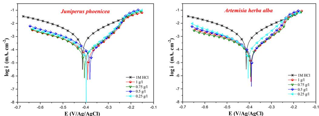
**Figure 2.** Polarization curves of mild steel in 1 M HCl in the presence of various concentrations of the *Juniperus phoenicea* and *Artemisia herba-alba* inhibitors.
