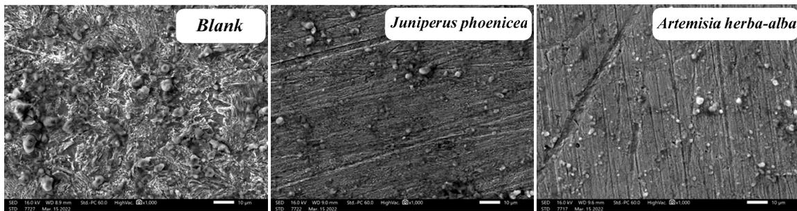
**Figure 7.** SEM images of mild steel after 6 h of immersion in 1 M HCl solution and in the presence of *Artemisia herba-alba* and *Juniperus phoenicea* inhibitors.
