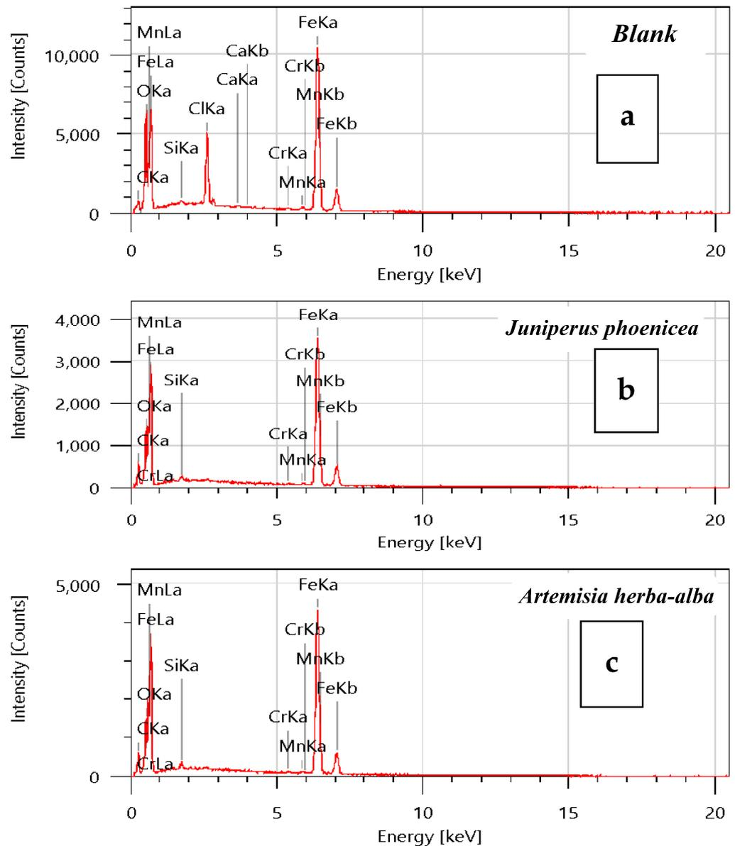
**Figure 8.** EDX spectra of mild steel after 6 h immersion in 1 M HCl solution (a) and in the presence of *Juniperus phoenicea* (b) *Artemisia herba-alba* (c).
