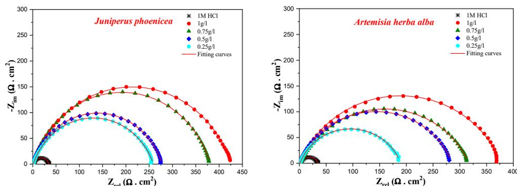
**Figure 3.** Impedance diagrams in the Nyquist plots of mild steel obtained in 1 M HCl in the presence of different concentrations of *Artemisia herba-alba* and *Juniperus phoenicea* inhibitors.
