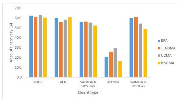
**Figure 1.** Evaluation of different elution solvents/solvent mixtures for the extraction of the target analytes. (BPA: Bisphenol A, BisGMA: bisphenol A methacrylate glycidate, TEGDMA: triethyleneglycol-dimethacrylate, UDMA: urethane dimethacrylate).
