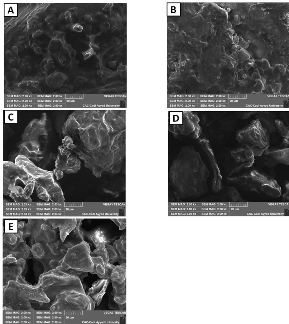
**Figure 2.** Scanning electron microscopy (SEM) images of different particle size classes. (A) >300 μm, (B) >125; ≤300 μm, (C) >50; ≤125 μm, (D) >25; ≤50 μm, (E) ≤25 μm.
