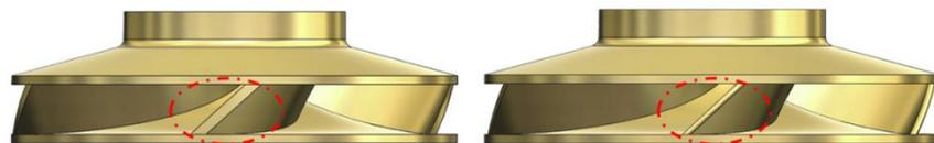
**Figure 2.** Physical picture of rounded blades.
