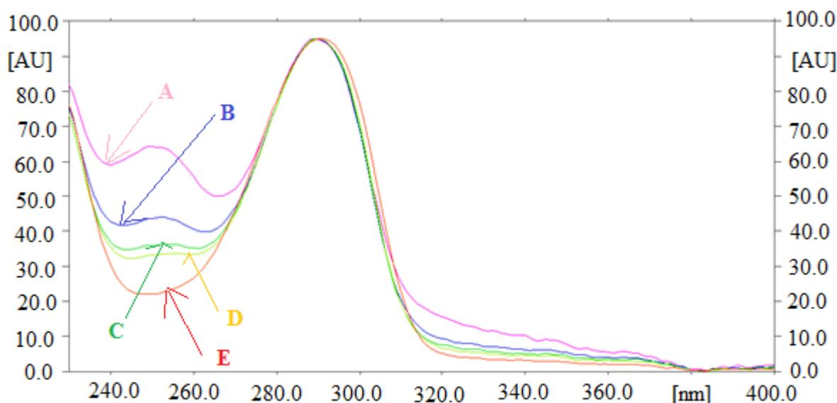
**Figure 2.** Overlaid ultraviolet (UV) absorption spectra of (A) standard HDQ, (B) commercial whitening cream (CWC) A, (C) CWC B, (D) CWC C, and (E) CWC D.
