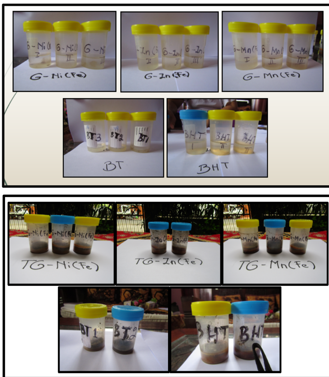
Figure 5. Filtrate and residue of soil after contamination (BT), after contamination and remediation by \text{H}_2\text{O}_2 (BHT), after contamination and remediation by the \text{H}_2\text{O}_2 -composite.
