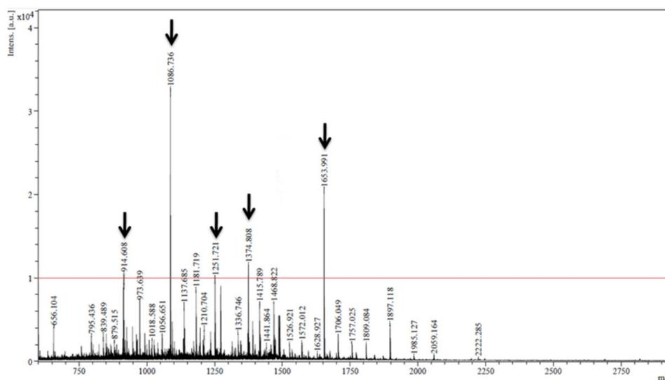
**Figure 2.** MALDI-ToF spectrum of the *B. bengalensis* protein hydrolysate of alcalase at 120 min. The arrows mark the peptides selected for the *de novo* sequencing. The red line across the spectrum marks the baseline intensity of  $1 \times 10^4$  a.u.
