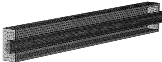
(c) Finite Element Model Cross Section
