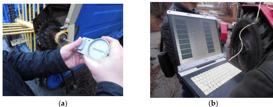
Figure 4. Determination of the rotation speed of the spreader working body shaft and the PTO shaft (a) and registering devices: PC and Oscill software (b) (for clarity and complete display of the drive and the working body, the protective barriers were dismantled at the time of photo-fixation).
