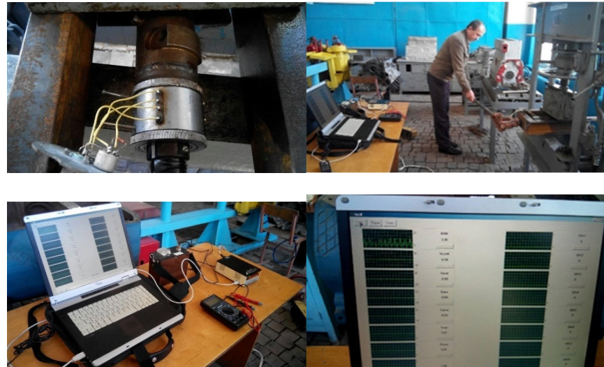
Figure 5. Calibration of mercury amalgamated current collector.
