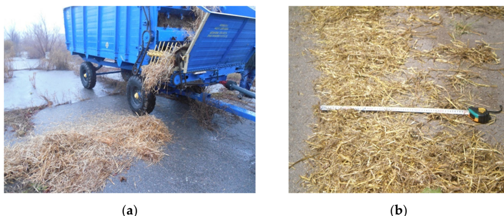
Figure 2. Determination of track length, passed by the mobile straw bedding spreader (a) and the spreading width (b).
