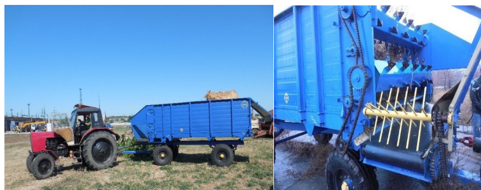
Figure 1. General view of equipment for the technological process of making straw bedding with rotary finger working bodies (for clarity and complete display of the drive and the working body, the protective barriers were dismantled at the time of photo-fixation).
