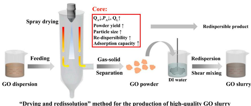
Figure 1. Graphic illustration of the “drying and redissolution” method for the production of high-quality GO slurry.
