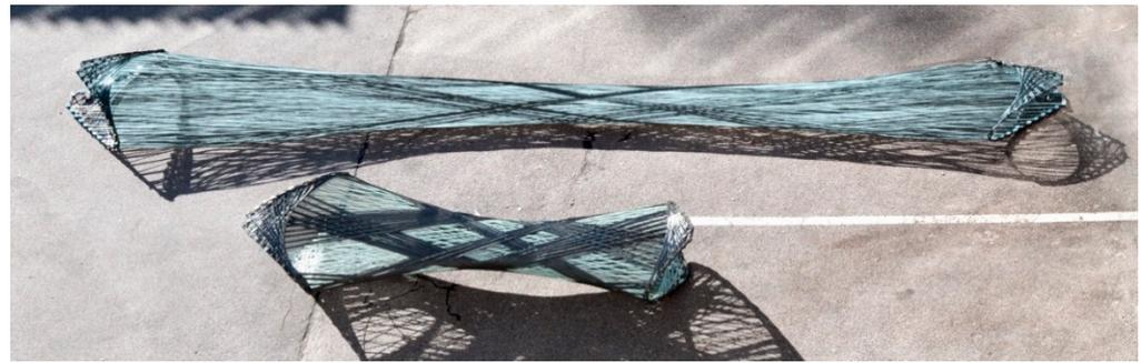
**Figure 5.** Fabricated research demonstrators. Big Fiber Component (**top**) and a BUGA-type state-of-the-art component (**bottom**).
