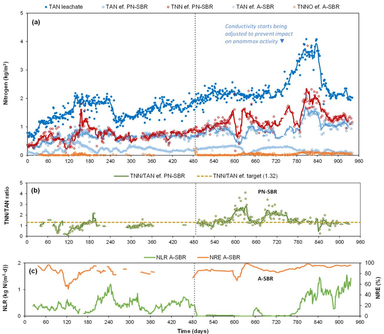
**Figure 6.** Performance of the full-scale system at the long-term; (a) Evolution of the concentration of the N species in both reactors (TAN: total ammonium N, TNN: total nitrite N, TNNO: TNN+ nitrate N); (b) TNN/TAN ratio in the PN-SBR effluent; (c) N loading rate and removal efficiency in A-SBR. Day 0 is 1 September 2017. The vertical dashed lines indicate when the landfill site stop receiving solid waste (on day 486).
