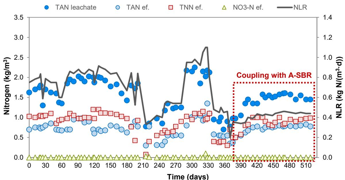
**Figure 3.** Long-term performance of the pilot-scale PN-SBR treating raw landfill leachate. By the end of the running period, PN-SBR was coupled with A-SBR (see Figure 4, *PHASE II-c*).
