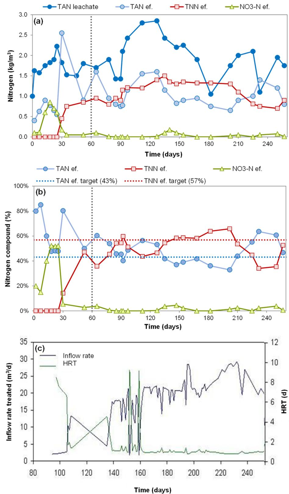
**Figure 5.** Performance of the full-scale PN-SBR during the start-up; (a) evolution of the concentration of the N compounds (TAN: total ammonium N, TNN: total nitrite N); (b) relative content of N compounds in the effluent; (c) inflow rate and hydraulic residence time (HRT) applied.
