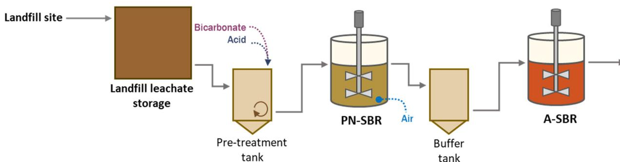
**Figure 1.** Descriptive scheme for the PANAMMOX<sup>®</sup> technology.
