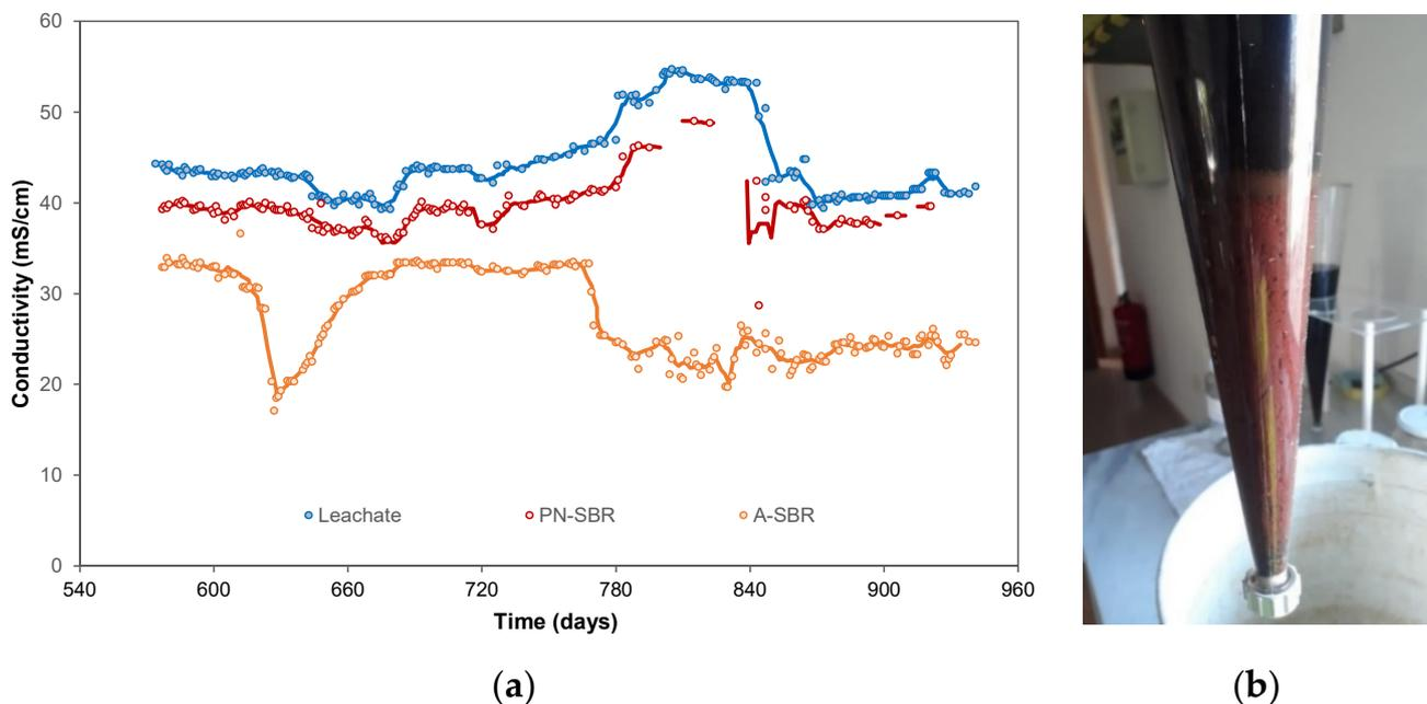
**Figure 7.** (a) Evolution of the conductivity in the treatment plant once the landfill site stopped receiving solid waste (day 486); (b) Detailed view of the biomass growing in A-SBR after decantation in an Imhoff cone (January 2020).
