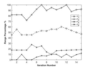
**Figure 13.** Trajectories of the process parameters of knowledge-informed simplex search based on historical gradient approximations (GK-SS) from  $X_1 = [202.73, 0.84, 7.82, 81.87]^T$ .
