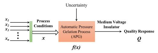
**Figure 1.** Relationship between the quality response of medium voltage insulators and the process conditions.
