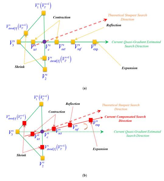
**Figure 8.** Optimization mechanisms of the simplex search method illustrated in a two-dimensional scenario. (a) Traditional simplex search method. (b) Revised simplex search method.
