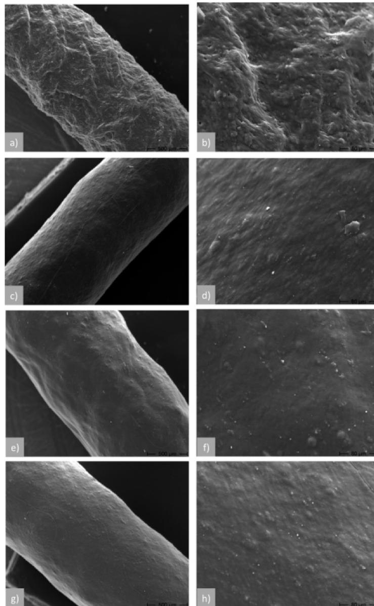
**Figure 4.** Surface of rice instant pasta processed at variable moisture content and screw speed: (a,b) 28%, 60 rpm; (c,d) 30%, 60 rpm; (e,f) 30%, 80 rpm; (g,h) 32%, 100 rpm; magnifications  $\times 100$  (left column) and  $\times 600$  (right column).
