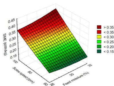
**Figure 3.** Specific mechanical energy (SME) as affected by feed moisture and screw speed during the processing of rice pasta.
