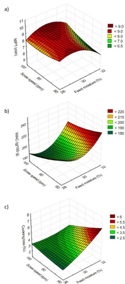
**Figure 1.** Minimum preparation time (MPT) (a), water absorption capacity (WAC) (b), and cooking loss (c) as affected by feed moisture and screw speed during the processing of rice pasta.
