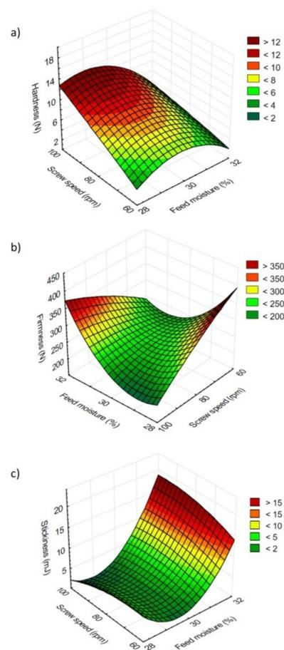
**Figure 2.** Hardness of dry pasta (a) as well as firmness (b) and stickiness (c) of hydrated pasta as affected by feed moisture and screw speed during the processing of rice pasta.
