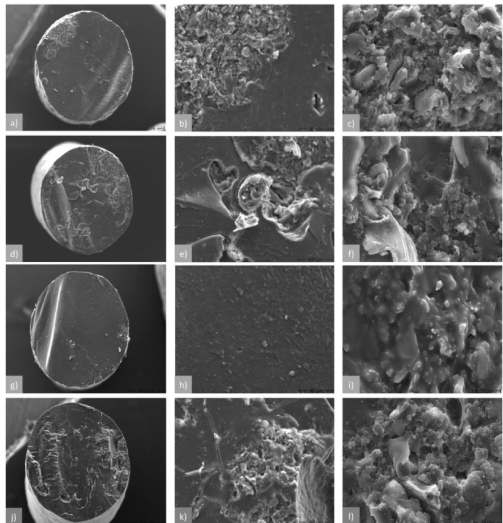
**Figure 5.** Cross-section of instant rice pasta processed at variable moisture content and screw speed: (a–c) 28%, 60 rpm; (d–f) 30%, 60 rpm; (g–i) 30%, 80 rpm; (j–l) 32%, 100 rpm; magnifications  $\times 125$  (left column),  $\times 600$  (middle column), and  $\times 2000$  (right column).
