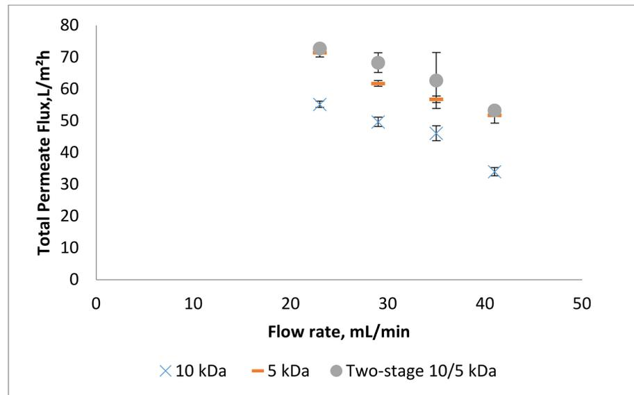
**Figure 3.** Total permeate flux at different feed flow rate for single and two stage ultrafiltration (UF) membrane.
