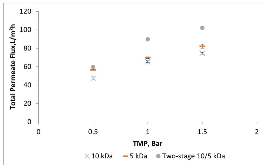
**Figure 5.** Total permeate flux at different trans-membrane pressures for single and two-stage UF membranes.
