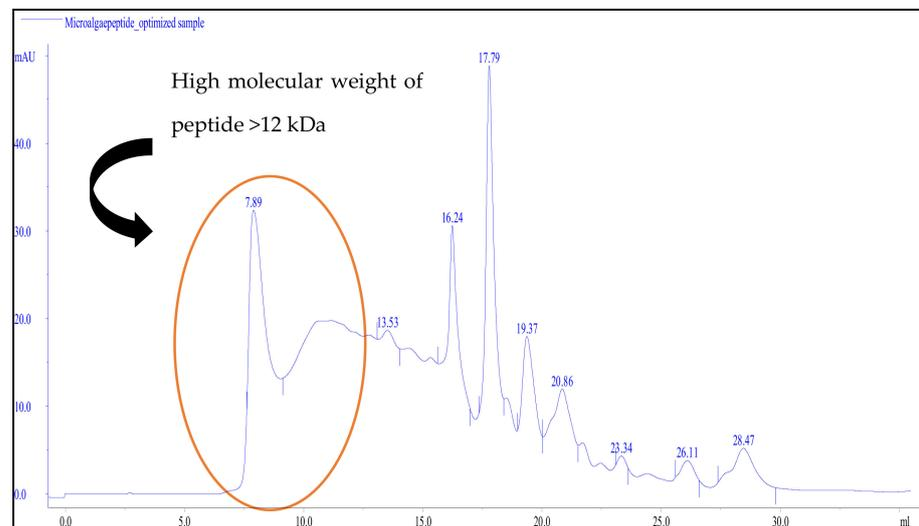
**Figure 11.** Fast Pressure Liquid Chromatography (FPLC) chromatogram of microalgae protein hydrolysate before fractionation using ultrafiltration membrane at a wavelength of 734 nm.
