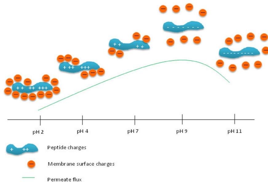
**Figure 8.** Schematic drawing of peptide structure and membrane surface state for single membrane.
