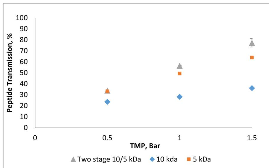
**Figure 6.** Peptide transmission at different trans-membrane pressure for single and two stage UF membrane.
