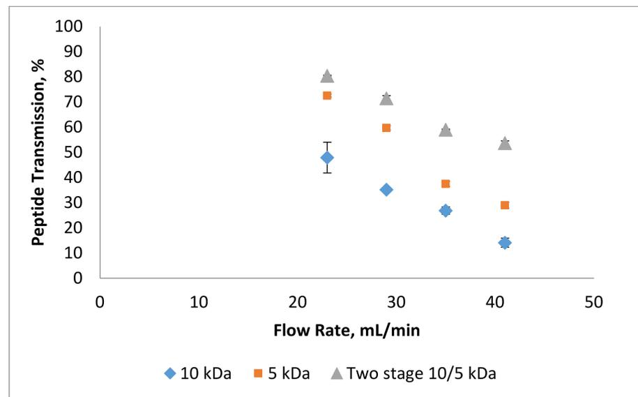
**Figure 4.** Peptide transmission at different feed flow rates for single and two stage UF membrane.
