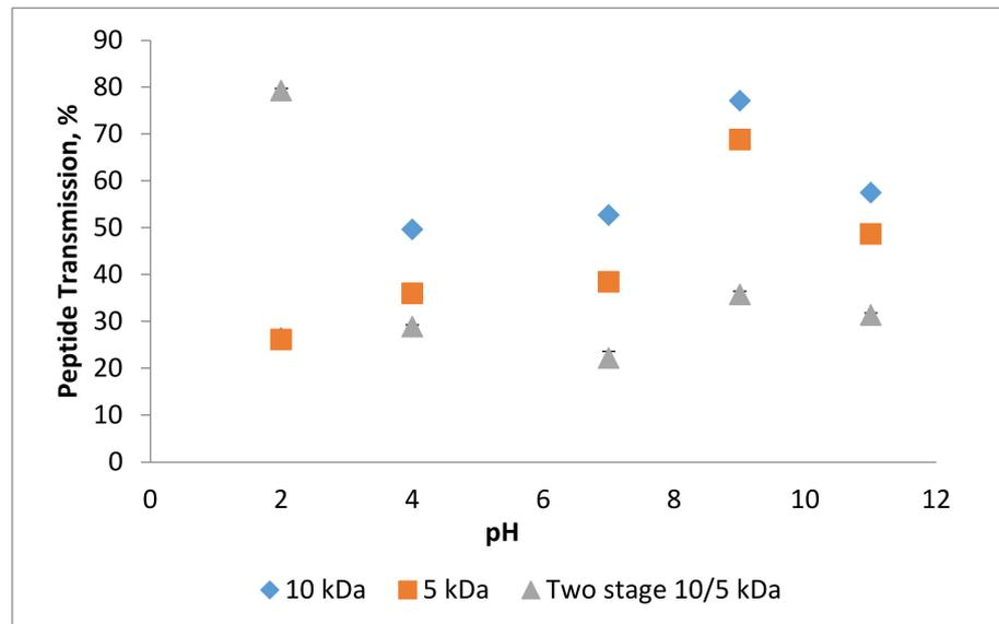
**Figure 10.** Peptide transmission at different pH for single and two stage UF membranes.
