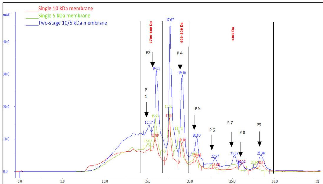
**Figure 12.** FPLC chromatogram of microalgae protein hydrolysate after fractionation using ultrafiltration membrane for single (10 and 5 kDa membrane) and two-stage 10/5 kDa membranes at a wavelength of 734 nm.
