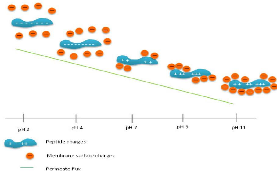
**Figure 9.** Schematic drawing of peptide structure and membrane surface state for the two-stage membrane.
