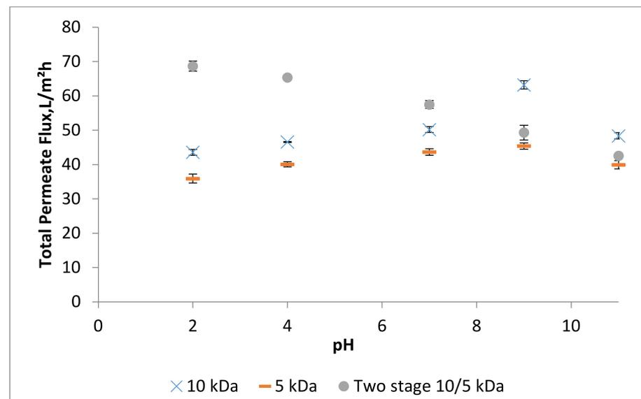
**Figure 7.** Total permeate flux at different pH for single and two stage UF membrane.
