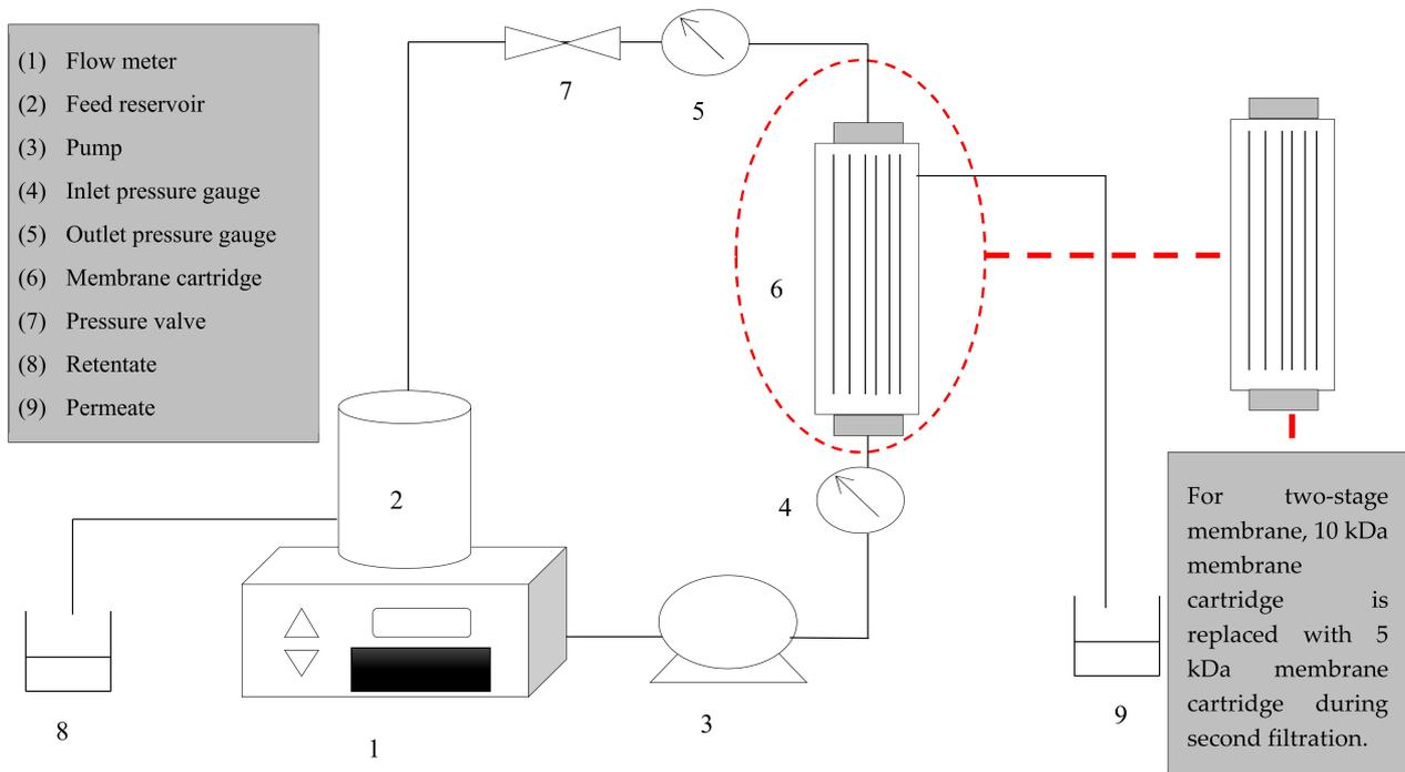
**Figure 1.** Schematic diagram of cross-flow ultrafiltration membrane.
