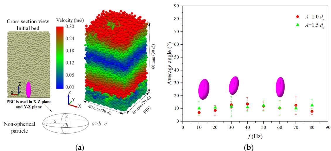
**Figure 1.** (a) Schematic of the simulated single non-spherical intruder in a vibrated bed of small particles; (b) average angle between the intruder’s long axis and the vibration direction—the error bar shows the variation range of the acute angle between the intruder’s long axis and the Z-axis.
