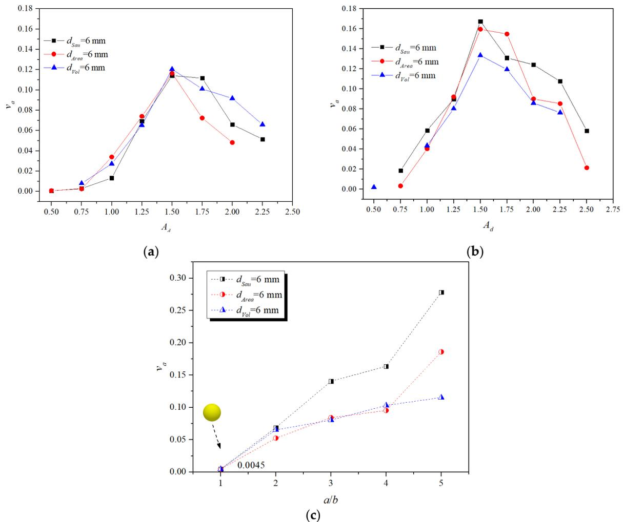
**Figure 4.** (a)  $v_a$  as a function of  $A$  with  $f = 20$  Hz and  $a/b = 2.0$ ; (b)  $v_a$  as a function of  $A$  with  $f = 20$  Hz and  $a/b = 3.0$ ; (c)  $v_a$  as a function of  $a/b$ , with  $f = 20$  Hz and  $A = 1.25 \cdot d_s$ . The yellow sphere means the intruder of  $a/b = 1.0$ .
