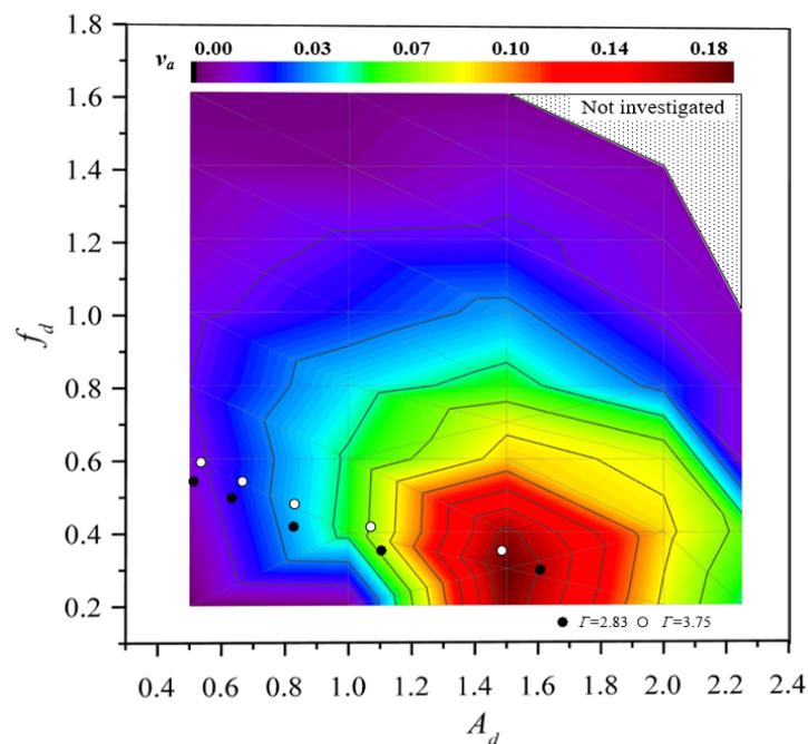
**Figure 10.**  $v_a$  as a function of  $f_d$  and  $A_d$  for the intruder of  $d_{Sau} = 6$  mm,  $a/b = 3.0$ .  $\circ$  and  $\bullet$  show the vibration conditions used in [31].
