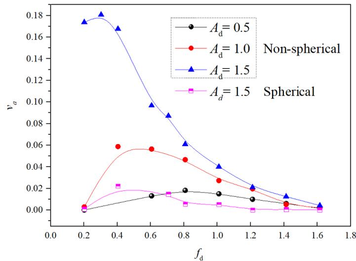
**Figure 7.** The influence of  $f_d$  on  $v_a$  for the spherical intruder ( $d_l = 6$  mm) and the non-spherical intruder ( $d_{S_{\text{intr}}} = 6$  mm,  $a/b = 3.0$ ).
