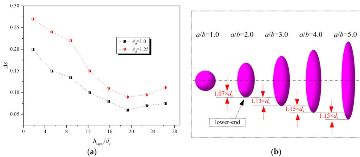
**Figure 6.** (a)  $\Delta\epsilon$  varies with bed layer; (b) a schematic of intruders with different aspect ratios.
