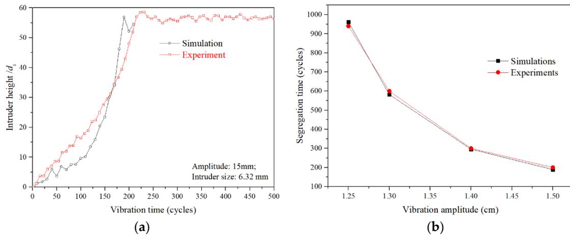
**Figure 2.** Comparison of simulation results and experiment results in Nahmad-Molinari et al. [11]: (a) the ascending height of the intruder as a function of vibration time; (b) the segregation time as a function of vibration amplitude under  $f = 7.5$  Hz.
