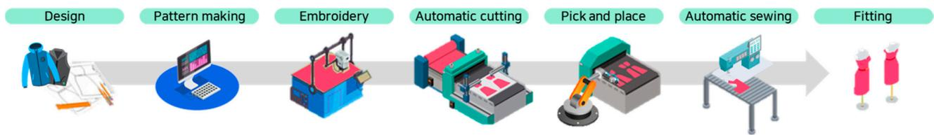
**Figure 6.** Automated manufacturing process for smart clothing.
