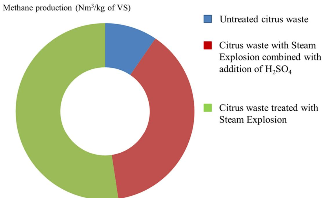
**Figure 3.** Methane production from citrus waste and comparison of results obtained from biomass untreated, and upon pre-treatment; steam-explosion (at 150 °C for 20 min), and steam-explosion combined with concentrated sulfuric acid (0.5% concentration, at 150 °C for 6 min). Adapted from [33].
