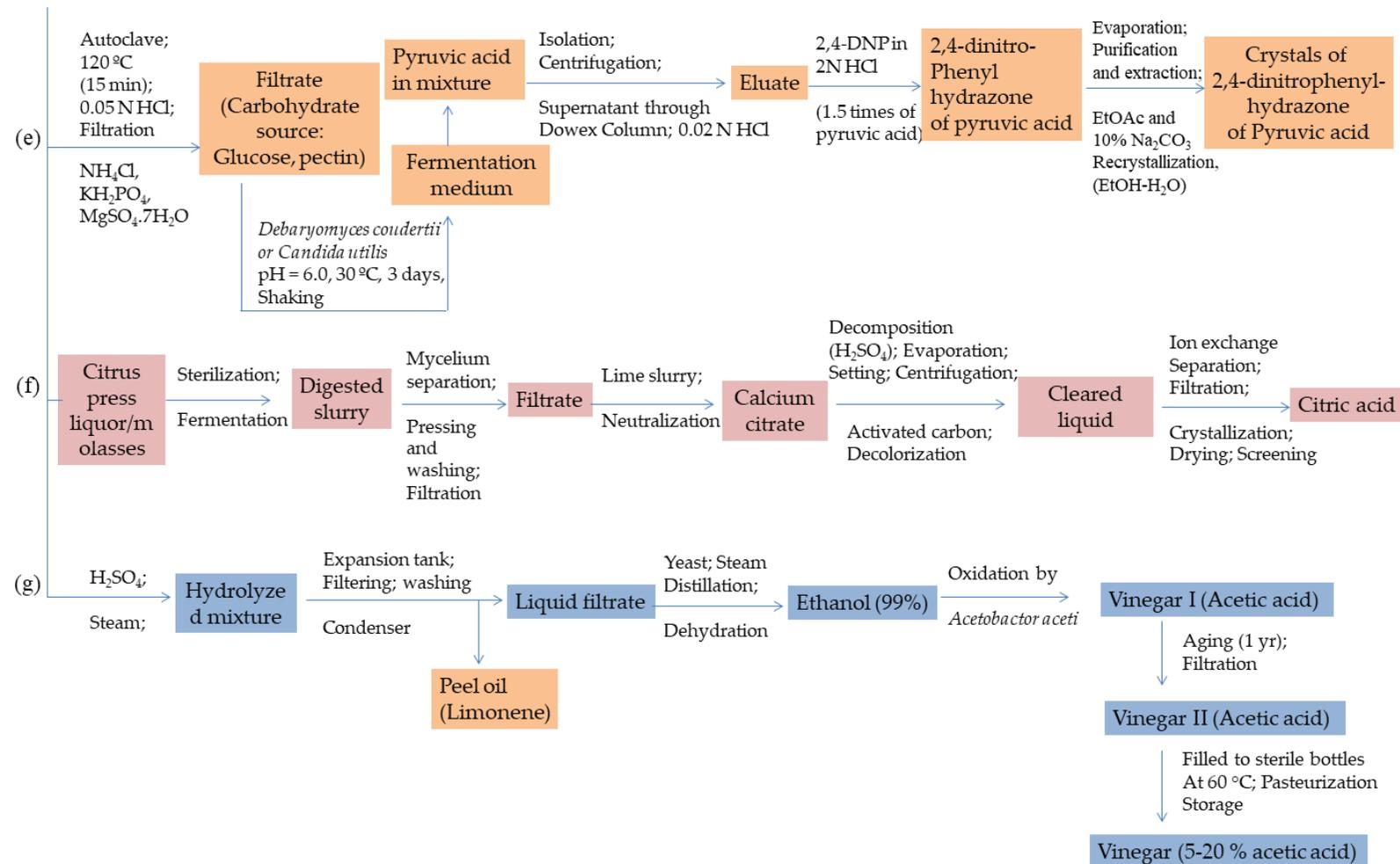
**Figure 11.** Steps involved in the production of organic acids, viz., (a) succinic acid (b), ascorbic acid (c), source material for vitamin-B complex (d) lactic acid (e) pyruvic acid, (f) citric acid, and (g) vinegar from processing of citrus waste.
