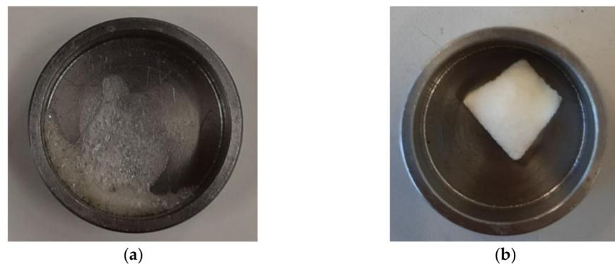
**Figure 5.** Macroscopic structure of electrospun PCL films after contact with scCO<sub>2</sub>: (a) not optimized and (b) optimized.
