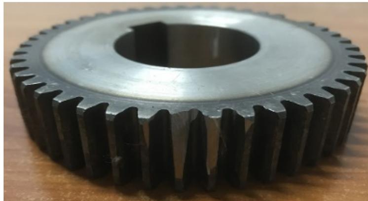
**Figure 2.** Partially broken mid-speed pinion gear.
