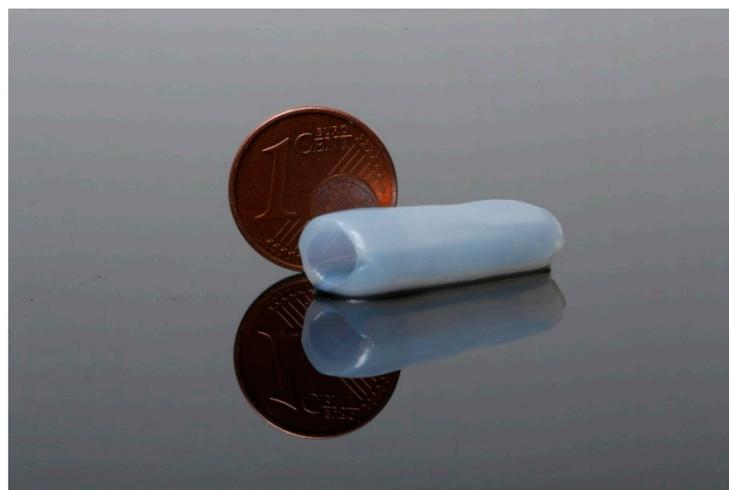
**Figure 1.** Photograph of a biocellulose tube (length: 50 mm, wall thickness: 1.5 mm), prepared according to variant 3 on a cylindrical bamboo template with a diameter of 5 mm. To visualize the size ratios of the biocellulose tube, it is placed next to a cent coin (© Andreas Heckel).
