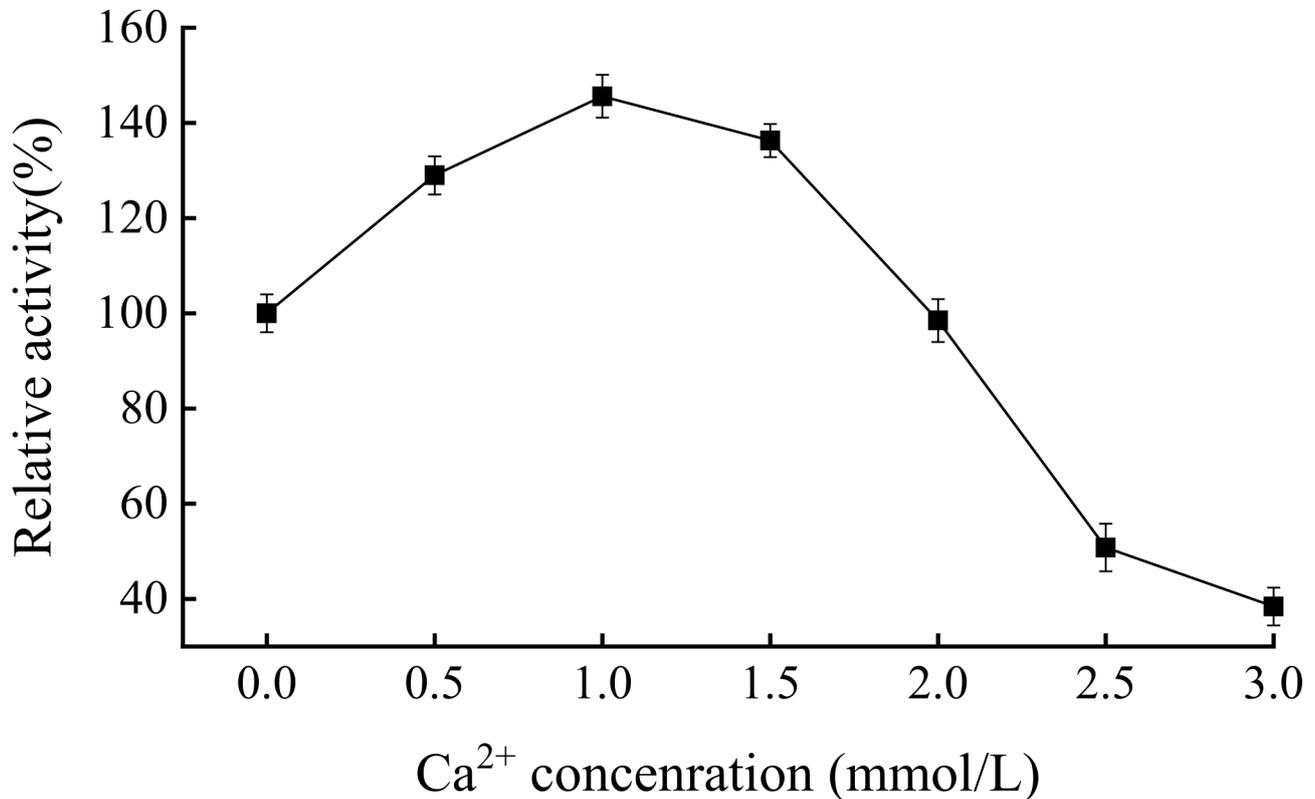
**Figure 6.** The effect of  $\text{Ca}^{2+}$  concentration on the relative activity of A129V. The pectate lyase activity without  $\text{Ca}^{2+}$  was taken as 100%. Values are the means  $\pm$ SD of three replicates.
