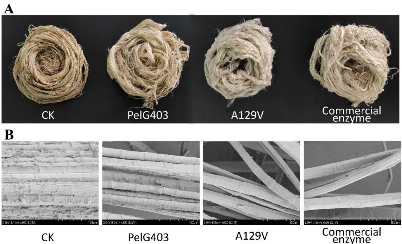
**Figure 7.** Surface morphology of the treated ramie. (A) Surface morphology of the untreated and treated ramie. (B) Scanning electron micrograph of the untreated and treated ramie.
