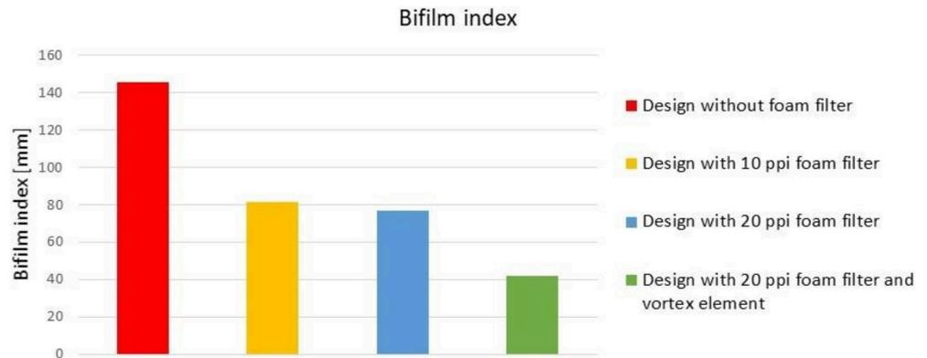
Figure 15. Results of bifilm index evaluation.
