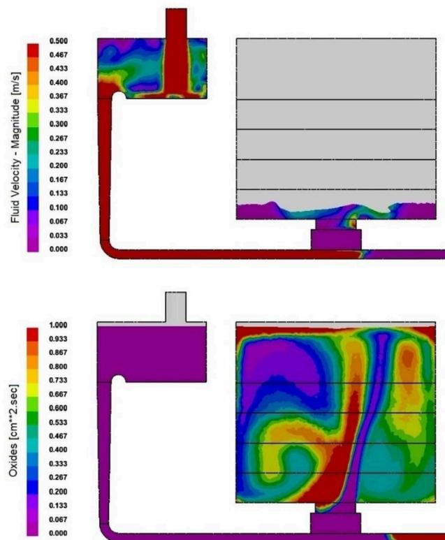
**Figure 6.** Simulations of the melt velocity and amount of oxides in the naturally pressurized gating system with 10 ppi foam filter.
