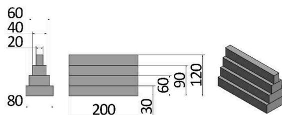
Figure 1. Casting design.
