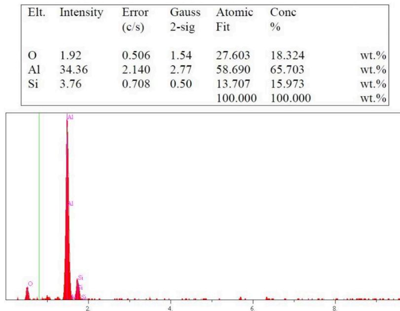
Figure 16. SEM and EDX analysis of pore inner surface.
