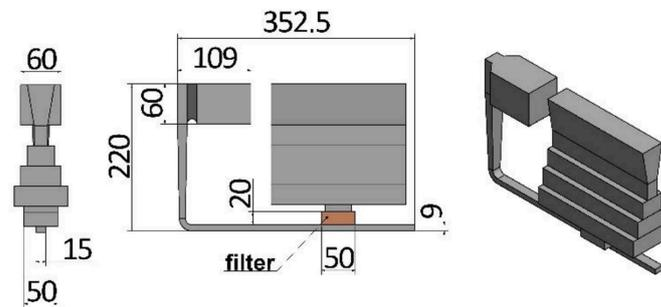
Figure 3. Naturally pressurized gating system with 10 and 20 ppi foam filter.
