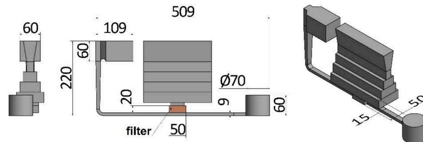
Figure 4. Naturally pressurized gating system with 20 ppi foam filter and vortex element.
