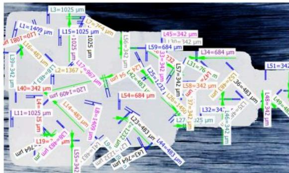
Figure 14. Bifilm index examination on the sample with 20 ppi foam filter and vortex element.
