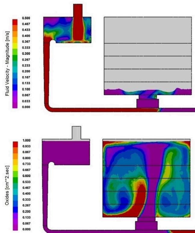
**Figure 7.** Simulations of the melt velocity and amount of oxides in the naturally pressurized gating system with 20 ppi foam filter.
