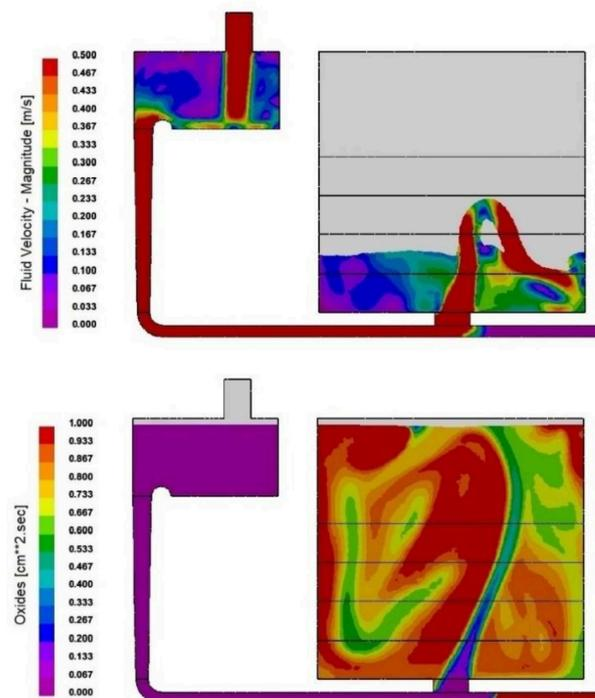
**Figure 5.** Simulations of the melt velocity and amount of oxides in the naturally pressurized gating system without foam filter.
