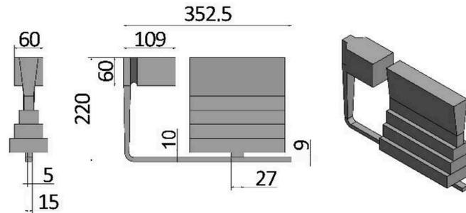
Figure 2. Naturally pressurized gating system without foam filter.
