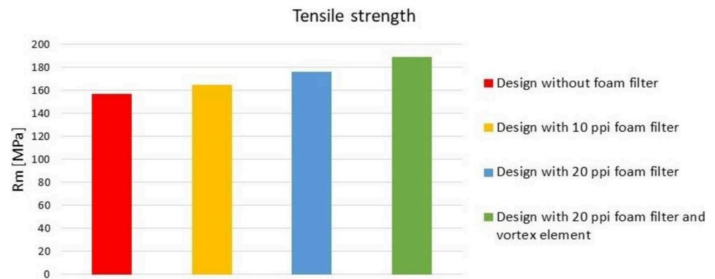
Figure 9. Results of tensile strength evaluation.
