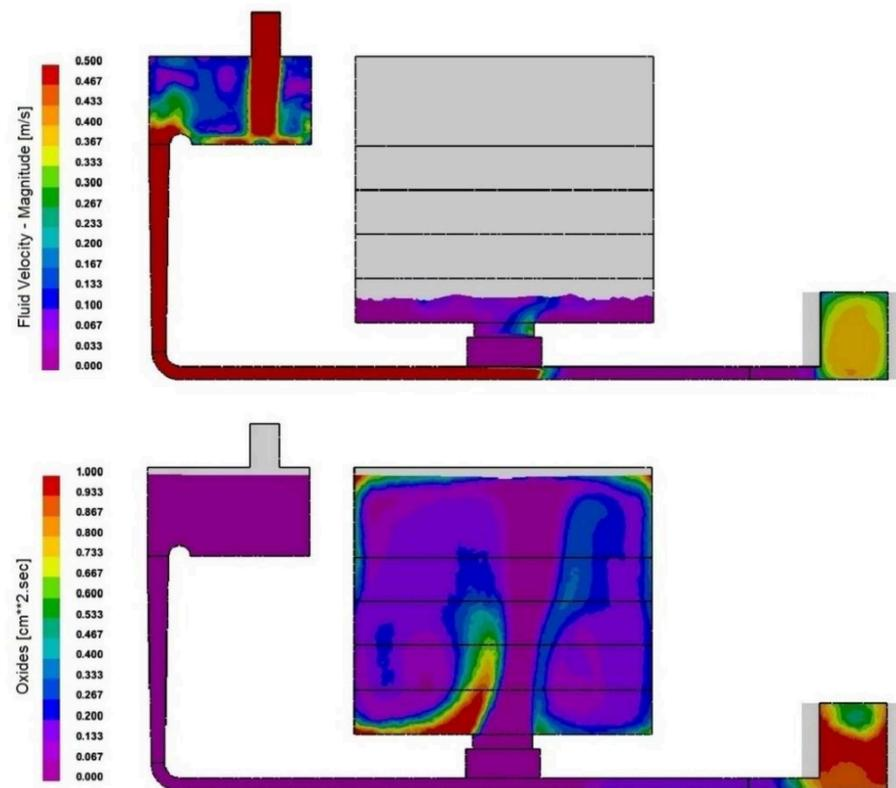
**Figure 8.** Simulations of the melt velocity and amount of oxides in the naturally pressurized gating system with 20 ppi foam filter and vortex element.
