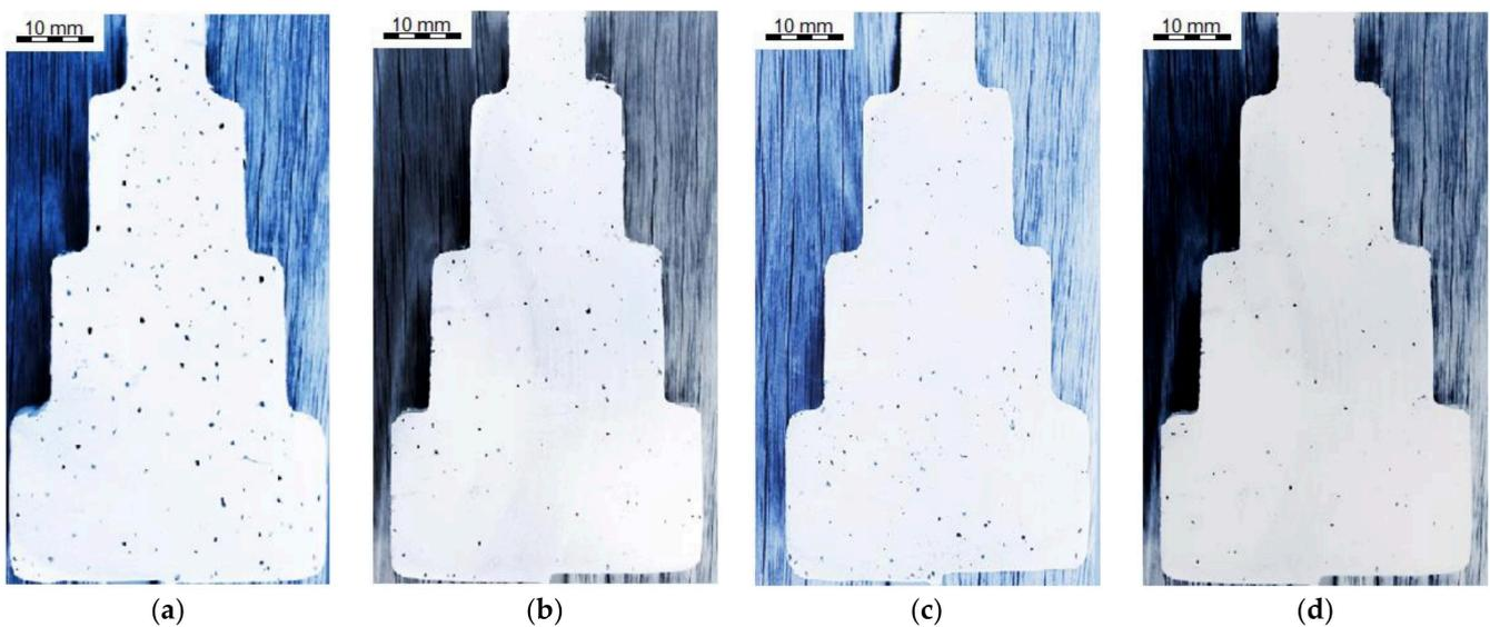
**Figure 12.** Porosity in specimens: (a) Design without foam filter; (b) Design with 10 ppi foam filter; (c) Design with 20 ppi foam filter; (d) Design with 20 ppi foam filter and vortex element.
