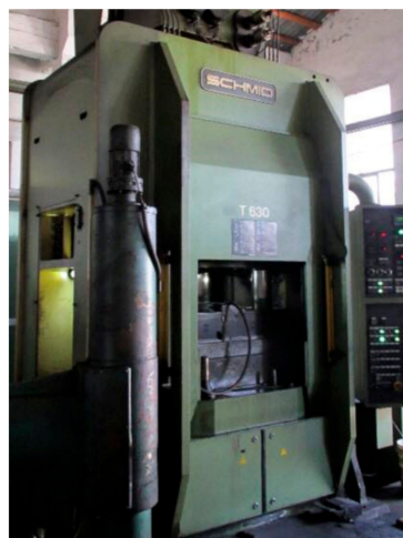
Figure 1. Structure (a) and equipment (b) of the 6300 KN cold orbital forging (COF) machine.
