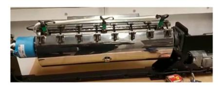
Figure 2. Torrefaction laboratory rotating batch reactor.
