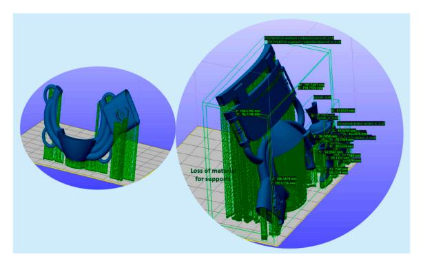
Figure 13. Diagram of the production of basic and advanced face caps using the stereolithography method.
