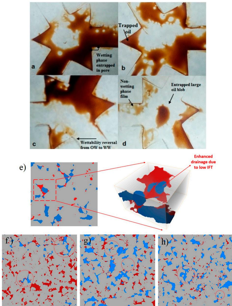
**Figure 7.** Digital microscope images of solution injection in the micromodel showing the pore-scale configuration and distribution of wetting and non-wetting phases within an initially preferential oil-wet medium for (a,b) surfactant solution and (c,d) surfactant and NP solution [60]; (e) 3D illustration of enhancement of the drainage process after a complex nanofluid injection and (f–h) 2D cross-sectional fluid occupancies for nanofluids in oil-wet systems [89].
