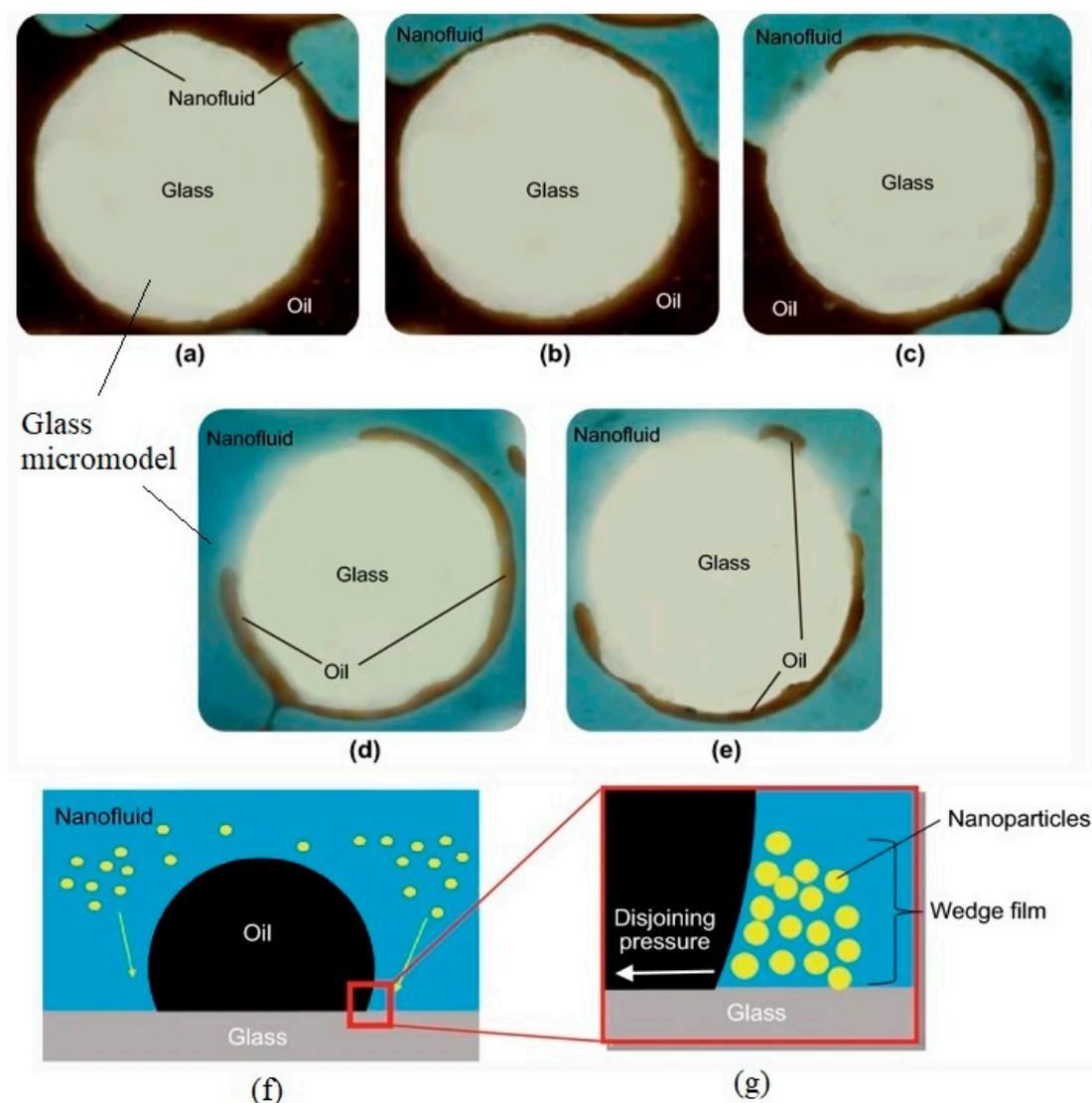
**Figure 8.** Surface wettability changes. Pore-scale views of the micromodel during nanofluid flooding for a period: (a) initial time, (b) 1000 s, (c) 2000 s, (d) 3000 s, (e) 5000 s of nanofluid injection; (f,g) illustration of oil droplet being loosened from the glass surface by adsorption of silica NPs [98].
