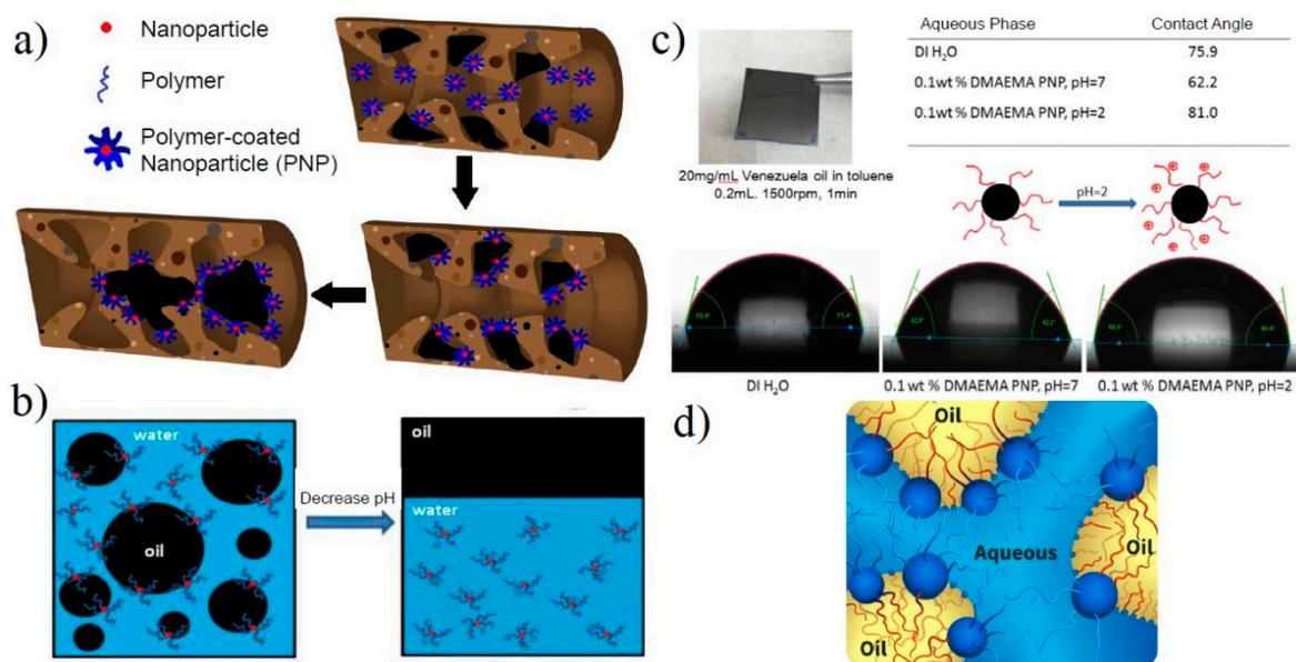
**Figure 4.** Schematic of (a) the use of polymer-coated NP additives to recover heavy oil trapped in porous media, (b) the demulsification of oil-in-water emulsions with changes in solution pH, (c) wettability alteration by polymer-coated NPs [40] and (d) schematic of oil–water microemulsion phases with polymer-coated NP additives [41].
