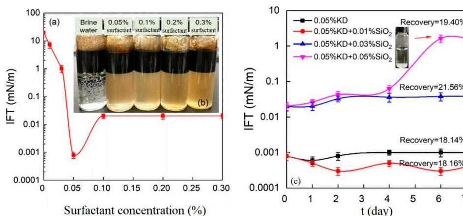
**Figure 6.** (a) IFT between surfactant solutions and oil at 80 °C, (b) emulsion stabilization image after 24 h at 80 °C and (c) IFT stability of surfactant-based nano-SiO<sub>2</sub> solutions at 80 °C [80].
