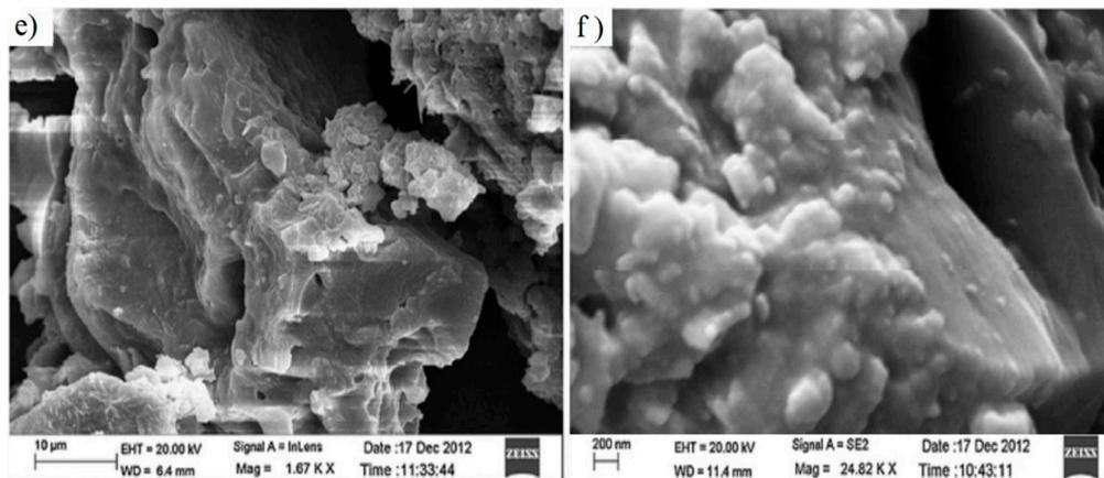
**Figure 5.** SEM images of sand samples with (a) 0.45 wt.% and (b) 0.90 wt.% clay NPs after polymer (c) Core sample before surfactant–polymer NP flooding, (d) deposition of NPs on the core sample after surfactant–polymer NP flooding [48]; (e,f) SEM images of core plug after flooding with NPs [36].
